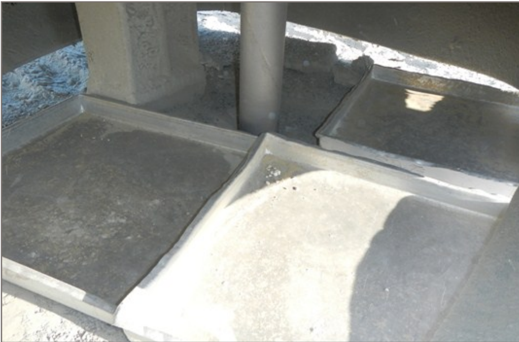
Photo 2: Metal containers underneath the curtain of the drill to collect soil samples.
