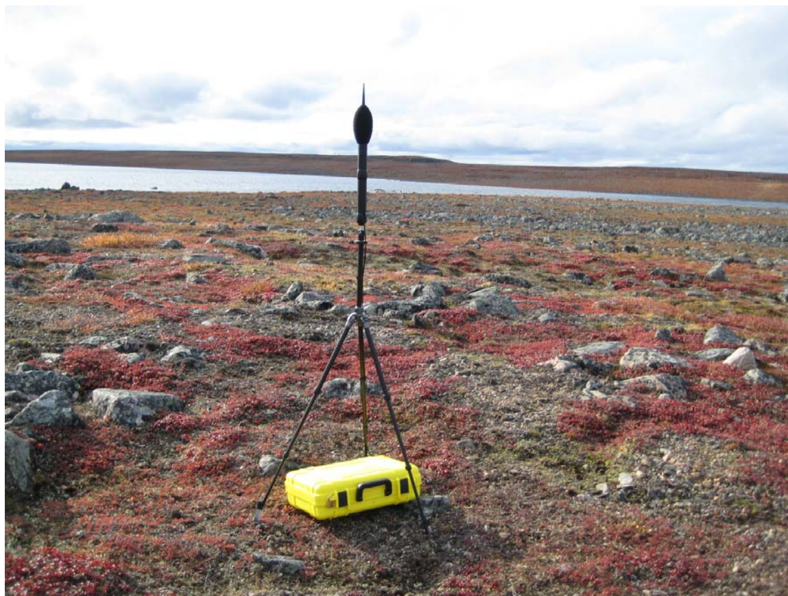
Photograph B.4 Future Mine Shop Area (R4) Noise Monitoring Setup (September 5 to 6, 2008)
