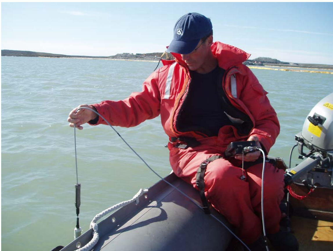
Photo 2-4. Analite turbidity probe in action.
