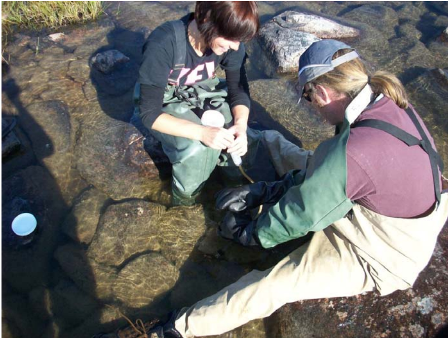
Photo D-1. Preparing the scrubber for removing periphyton from a rock.
