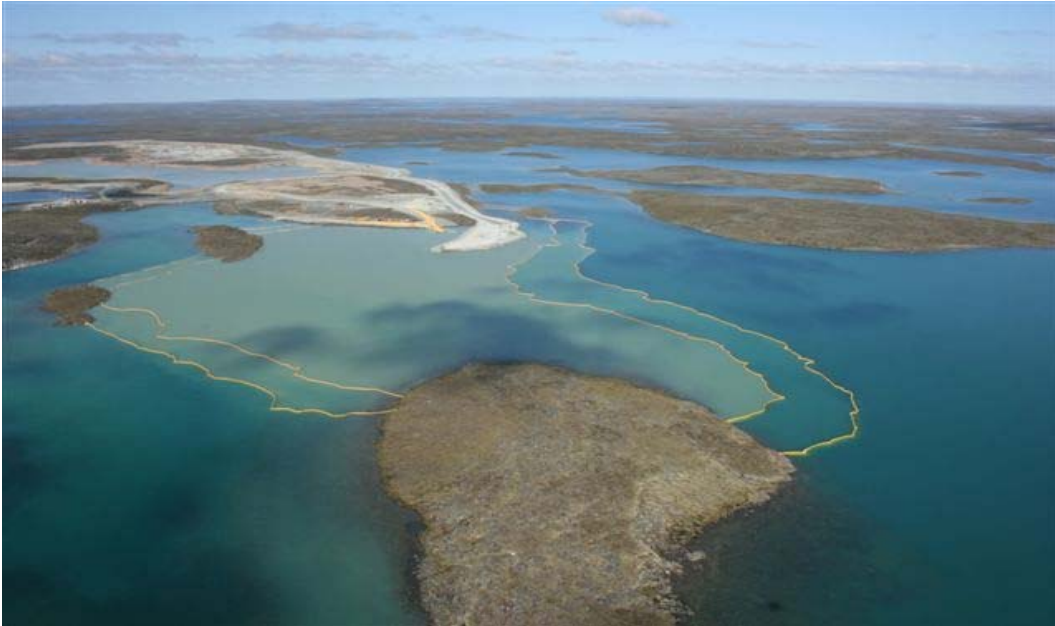
Photo 3-5. Elevated TSS within Bay-Goose Dike turbidity barriers, 14 August 2009 (Day 18).
