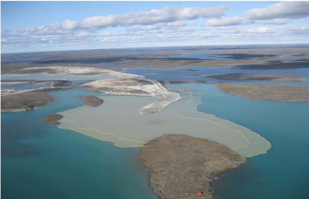
Photo 3-5. Elevated TSS within Bay-Goose Dike turbidity barriers, 14 August 2009 (Day 18).
