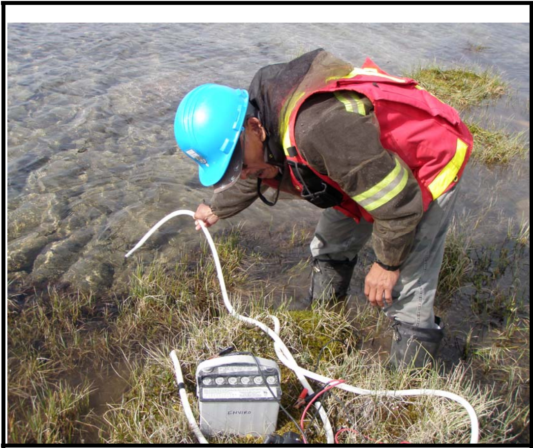
Photo No 7 : Water sampling using a small battery operated bilge pump and Teflon lined tubing
