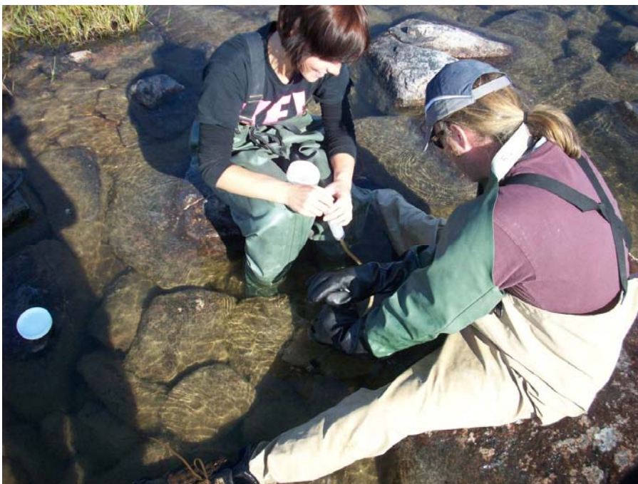
Photo D-5. Preparing the scrubber for removing periphyton from a rock.
