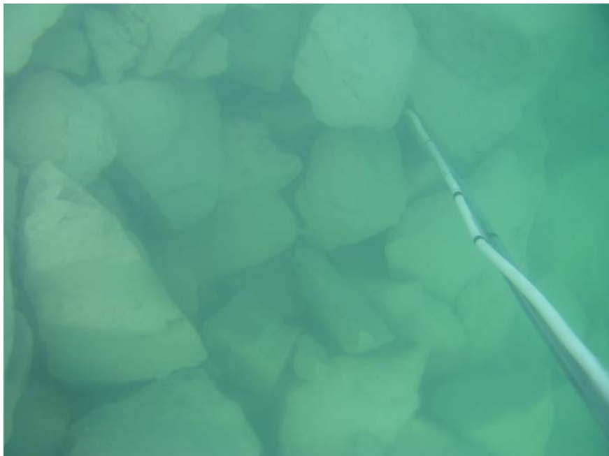
Photo A-3. A pole (4 m), with attached tube positioned between rocks of the East Dike, collected interstitial pore water.
