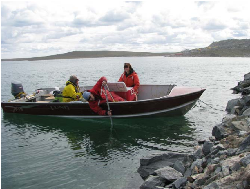
Photo A-2. Boat anchored to East Dike while placing pole with attached tube into interstitial space between rocks.
