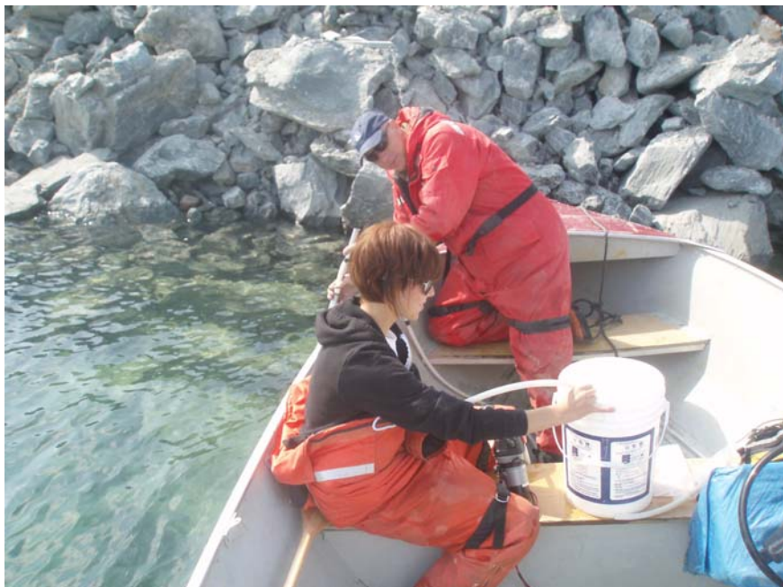
Photo A-4. Interstitial pore water collection into a HDSV bucket for subsequent decanting into sampling containers.
