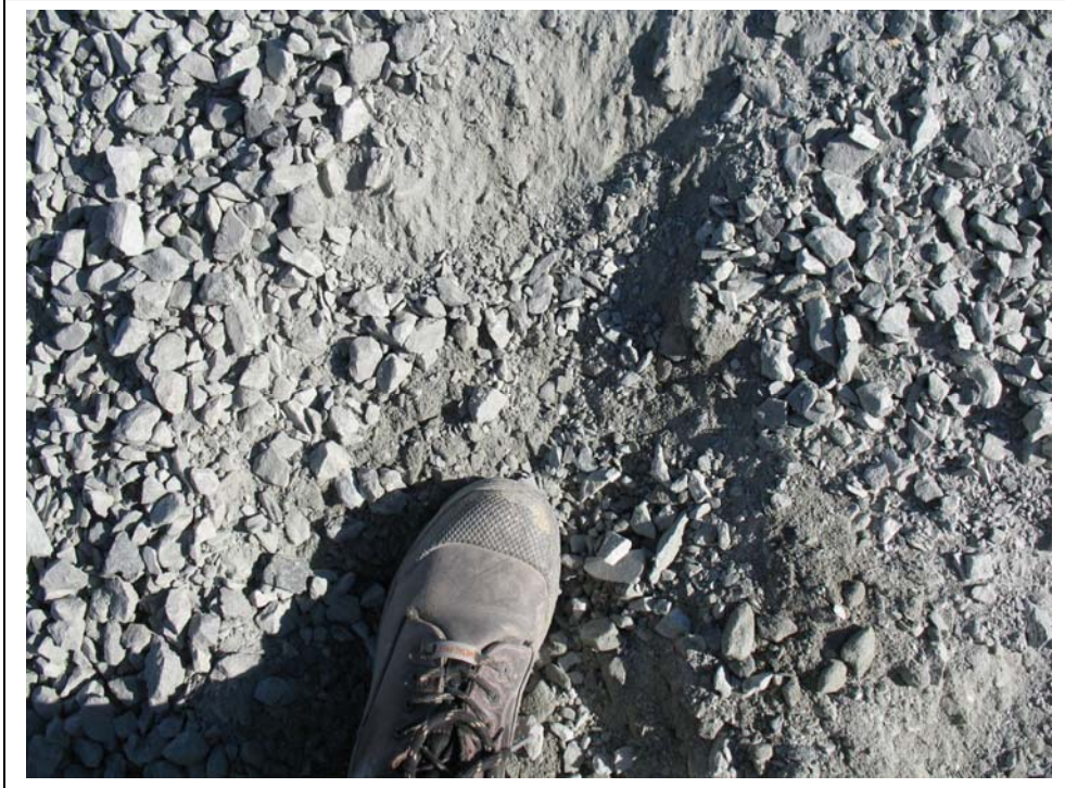
Photo # 9 Stormwater dike, stockpile of bedding material from PAG rock
