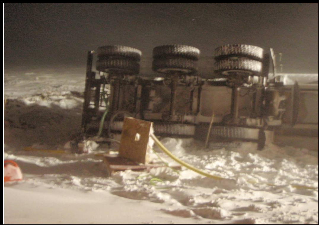
Photo No 1: 40,027L fuel truck flipped on its side; fuel transfer pumps in foreground; note poor visibility
