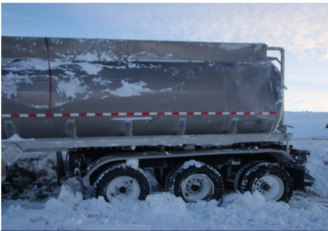
Photo No 12 : Dents at rear of the tanker; no punctures
