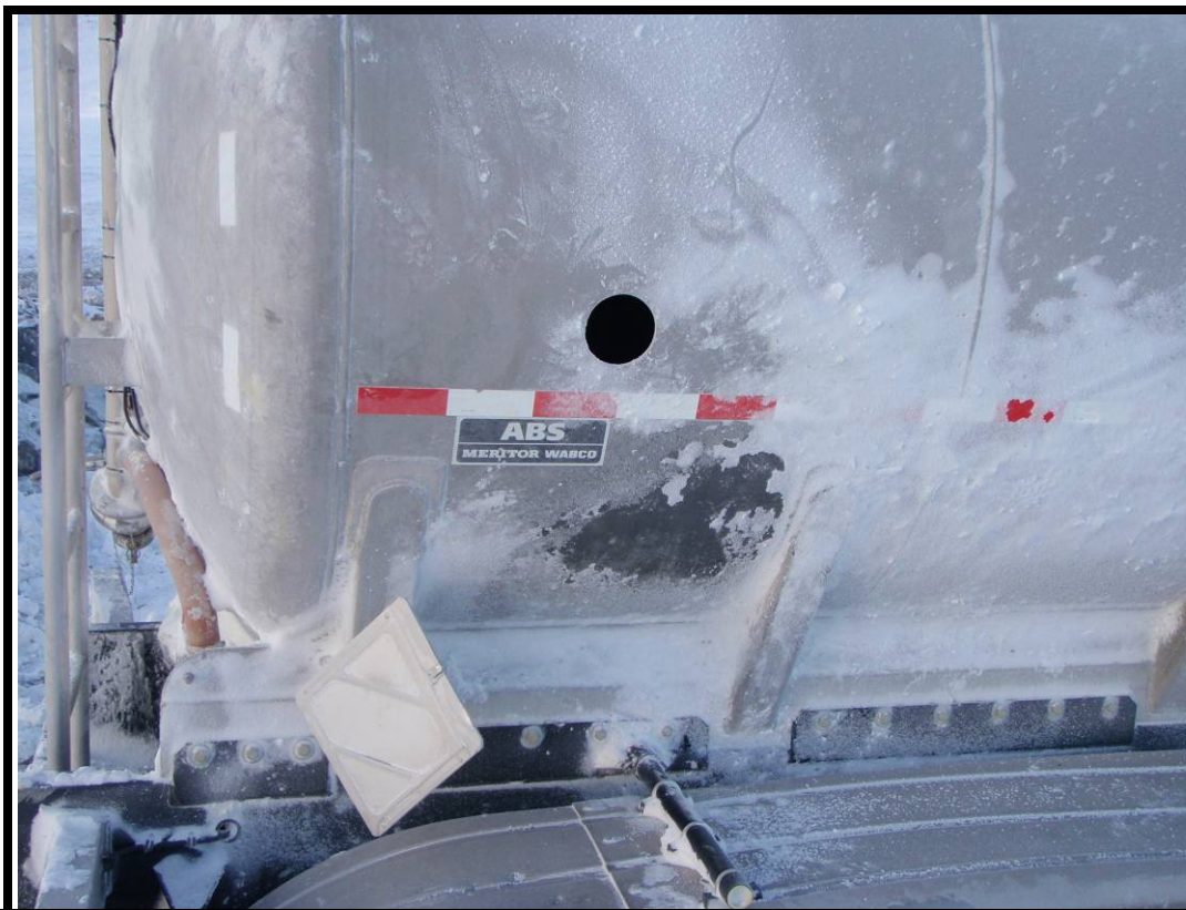
Photo No 13 : Drilled hole used to pump and recover fuel.
