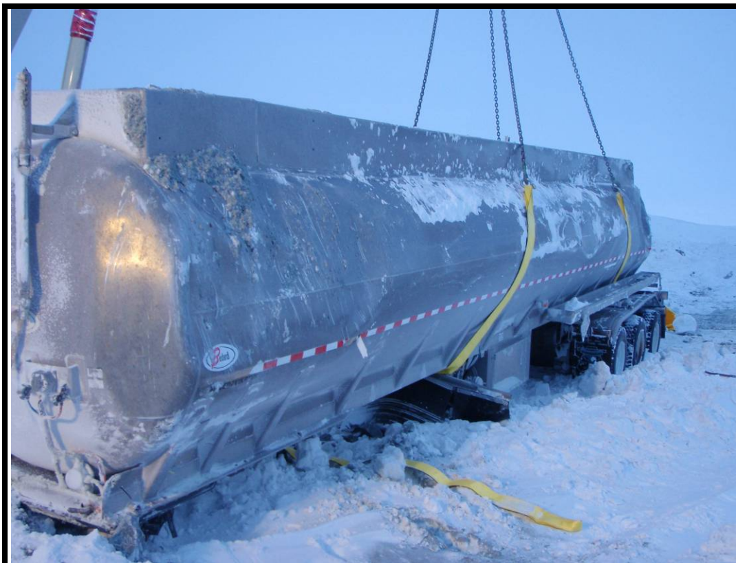
Photo No 11 : Dents at front of tanker
