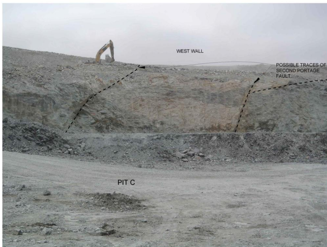
Photograph 15: Possible intersection of Second Portage Fault with west wall of Pit C
