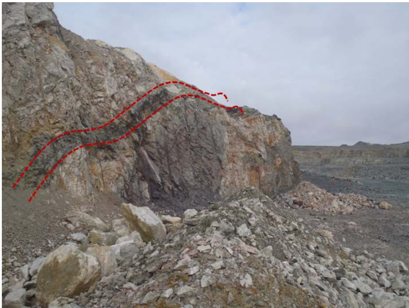
Photograph 8: Pit B west wall fault exposed in the 5116 bench face in 2011
