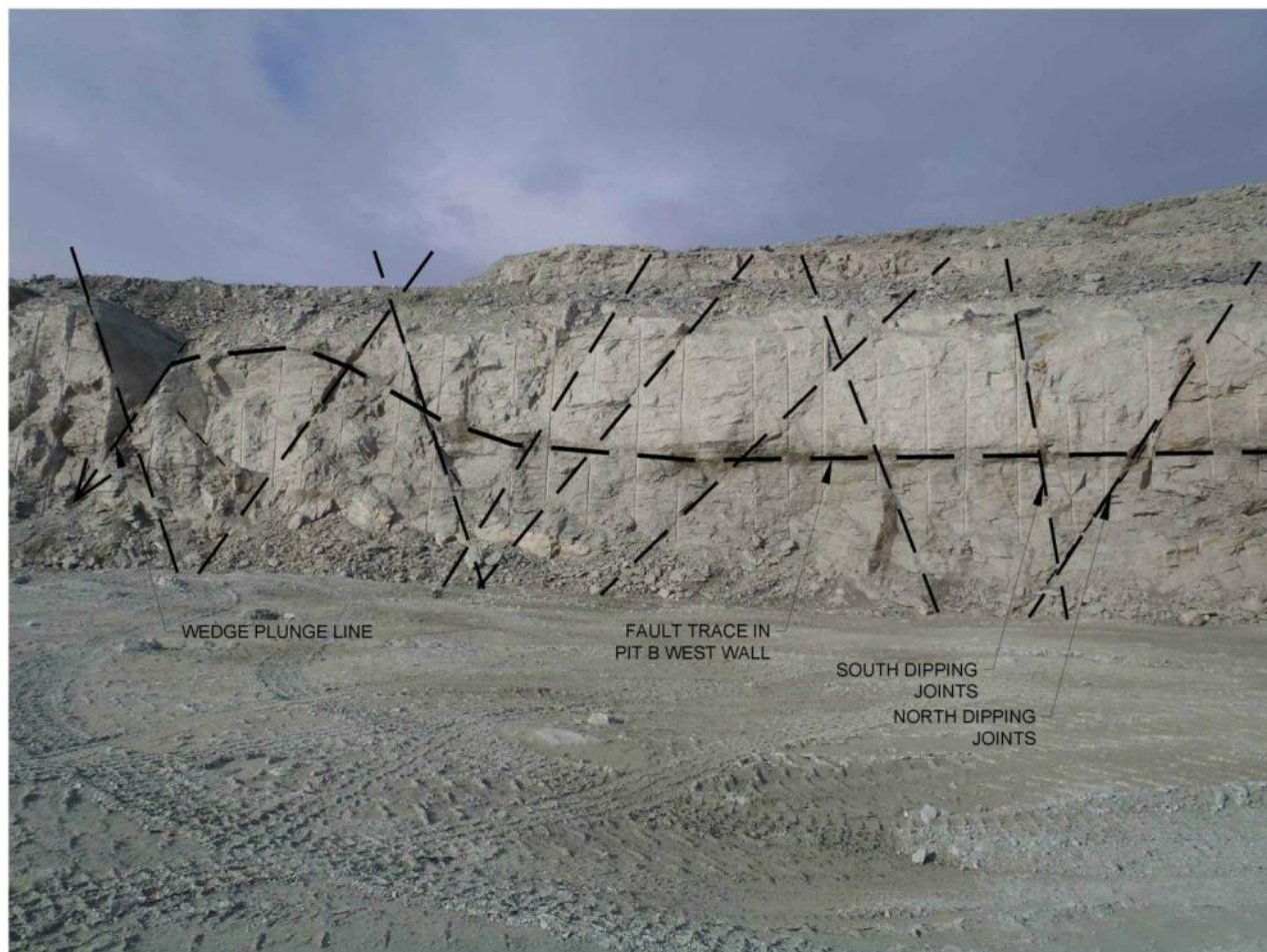
Photograph 11: Small-scale wedge structure noted in west wall of Pit B (viewed from Stop 5 in Figure 5)
