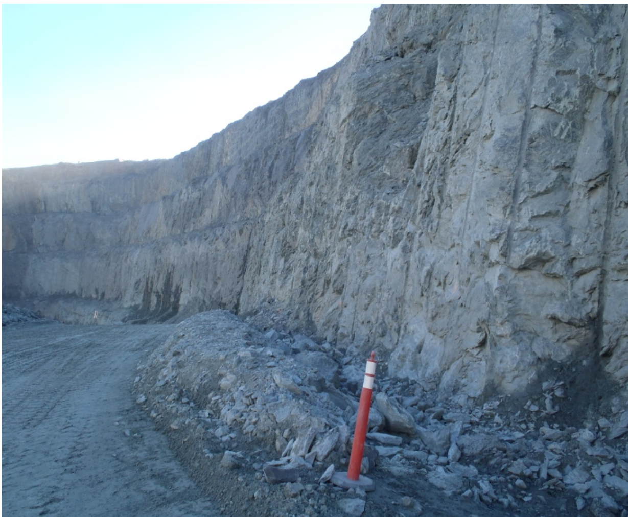
Photograph 25: Scallop-type structure in west wall of Pit E, adjacent to ramp and showing additional containment berm at toe of bench
