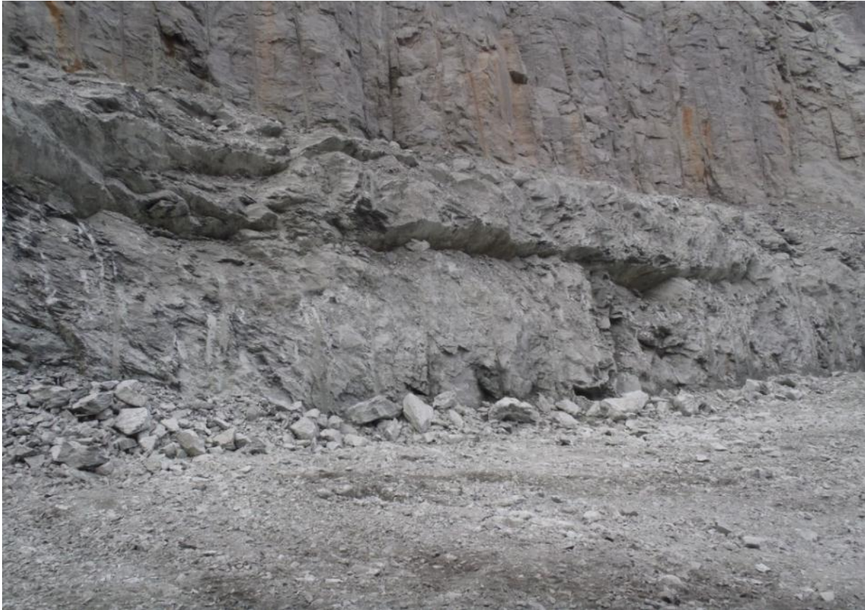
Photograph 23: Over-digging of ultramafic rock leading to overhangs (Stop 12 in Figure 5)
