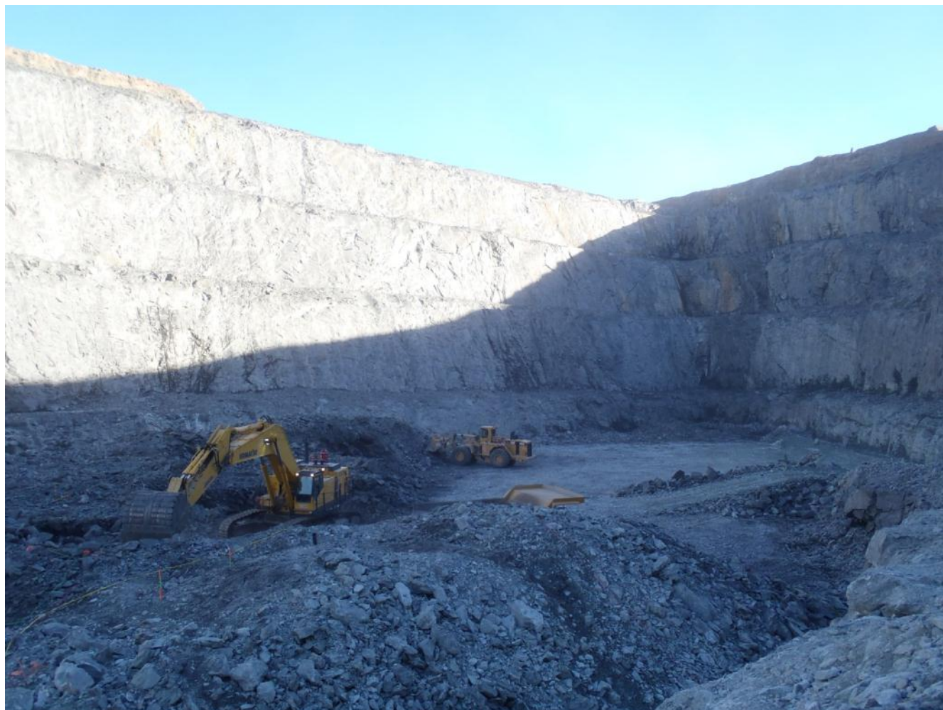
Photograph 27: East and southeast wall of Pit E showing generally good bench performance
