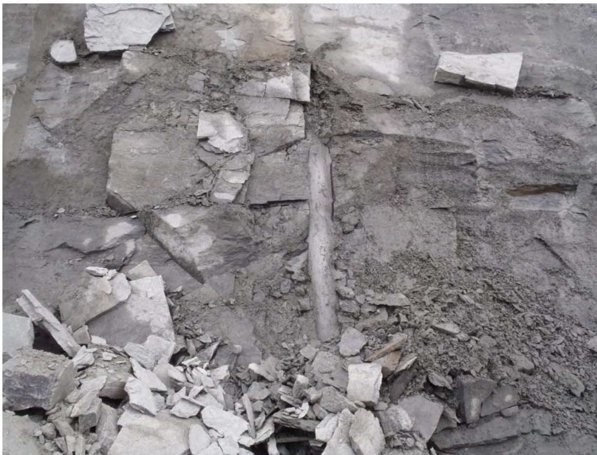
Photograph 39: Ice in blast holes near the south end of the current Goose Pit (Stop 6 in Figure 8)
