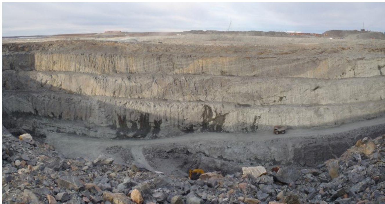
Photograph 22: Pit E viewed from above showing the generally good performance of the west wall (viewed from Stop 10 in Figure 5)
