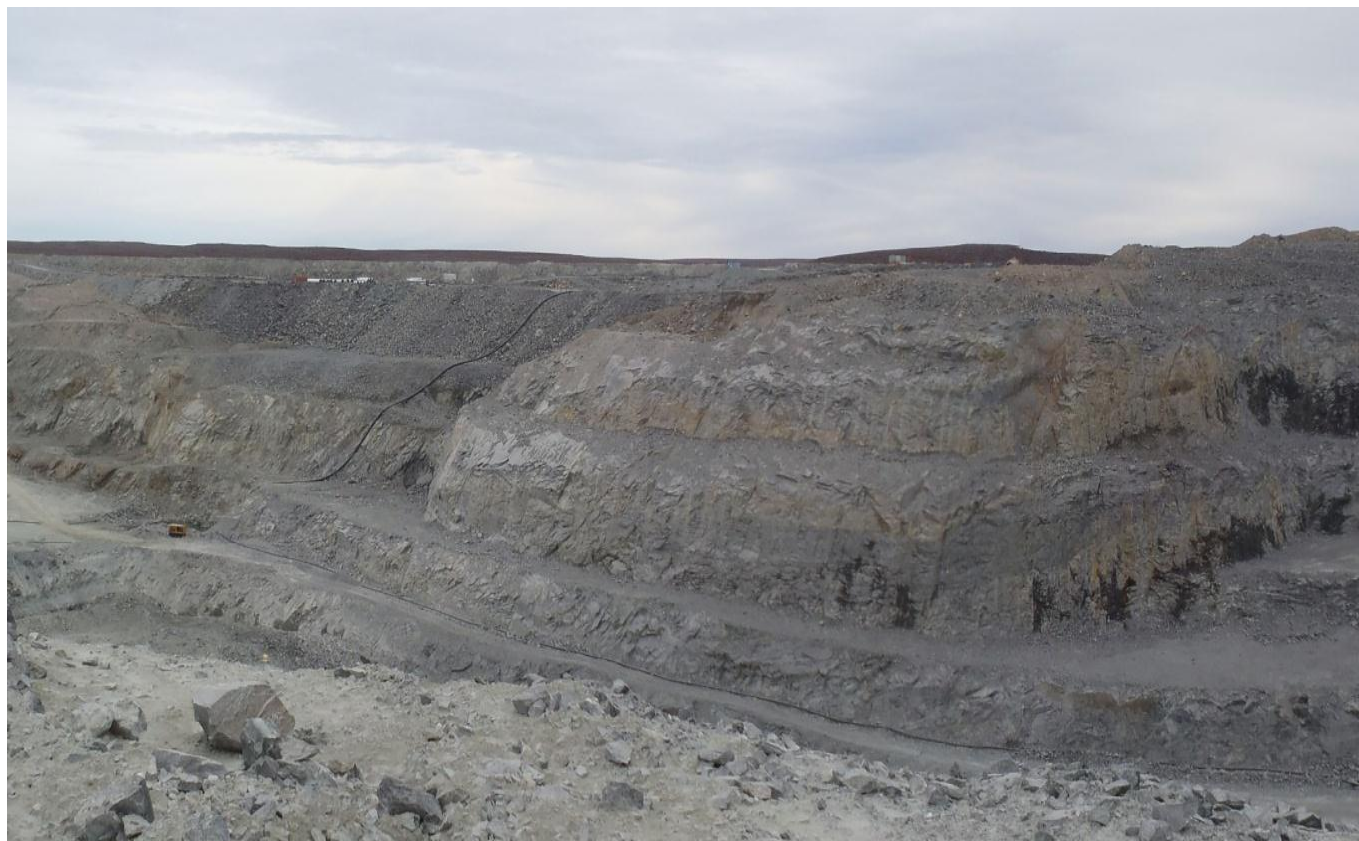
Photograph 19: North end of Pit D east wall showing undercut foliation and area of catchment loss, looking northeast (from Stops 7 and 8 in Figure 5)
