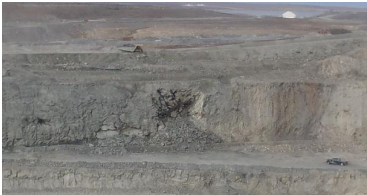
Photograph 3: Rock fall on west wall of Pit A on 5109/5123 bench, Stop 2 in Figure 5 (pickup truck in foreground is at 5,109 RL)
