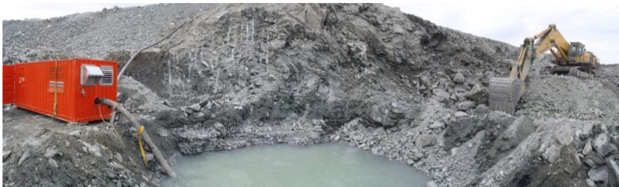
Photograph 40: Location of inflow in the South Goose Pit showing irregularly foliation and highly fissile material
