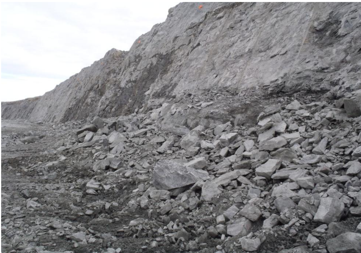
Photograph 31: Hard toes at 5,116 RL, Goose Pit east wall
