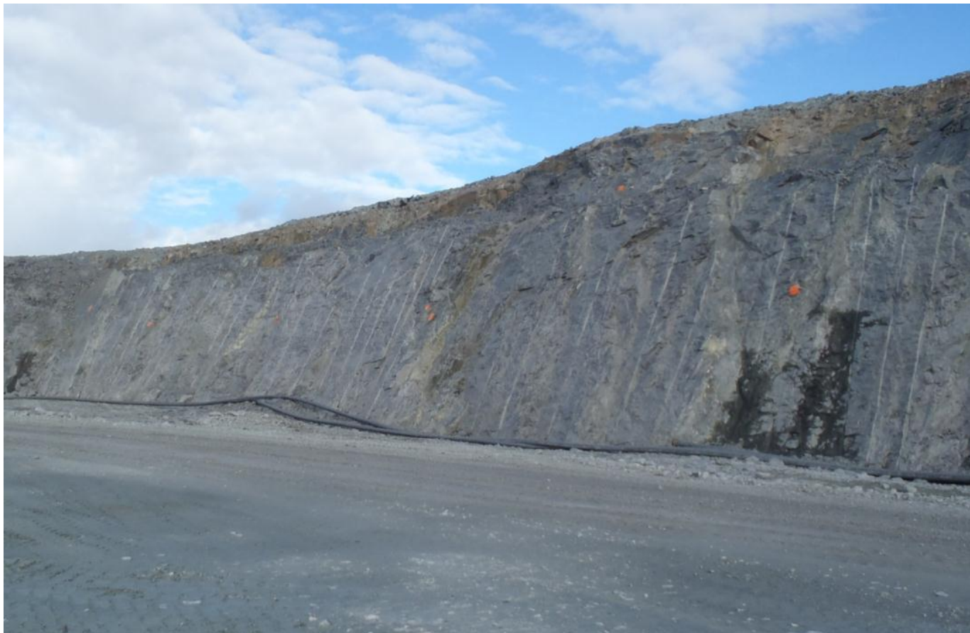
Photograph 36: East wall of Goose Pit showing prism density
