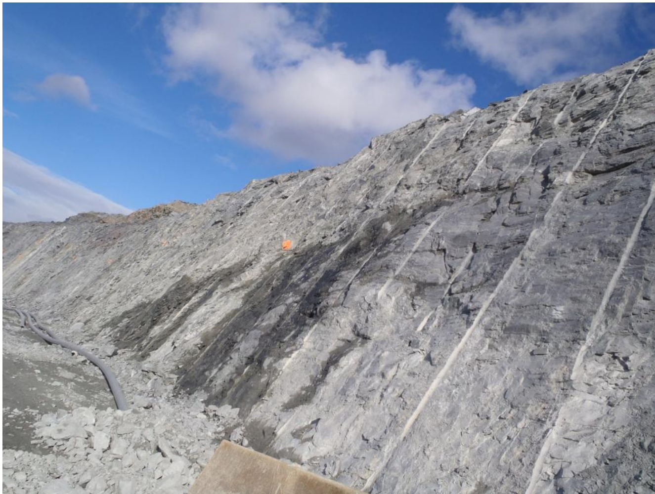
Photograph 30: East wall of Goose Pit showing pre-shear half barrels and west dipping foliation
