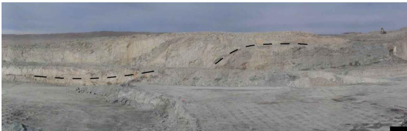
Photograph 9: Pit B west wall showing the exposure of the fault in the lower bench
