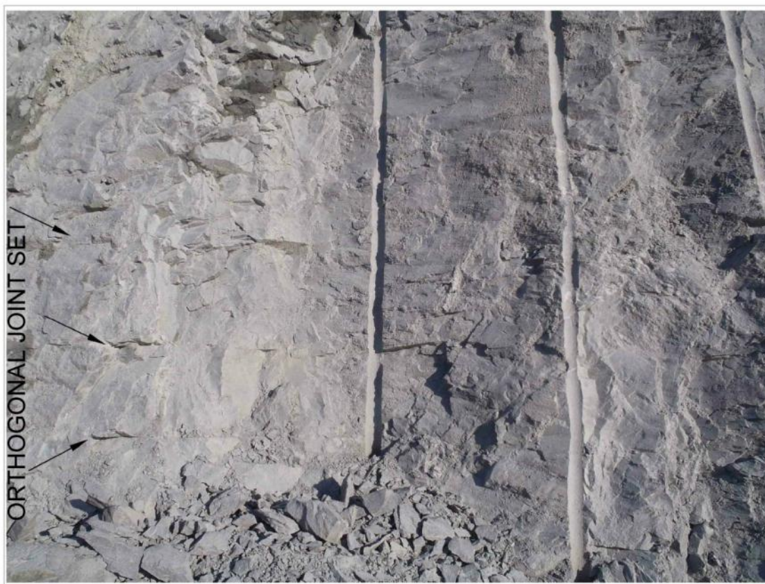
Photograph 37: Continuous orthogonal joint in the east wall showing significant rock bridging
