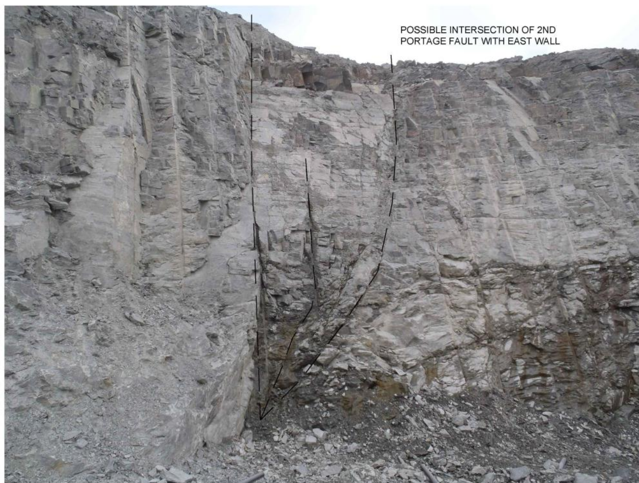
Photograph 14: Possible intersection of Second Portage Fault with east wall of Pit C
