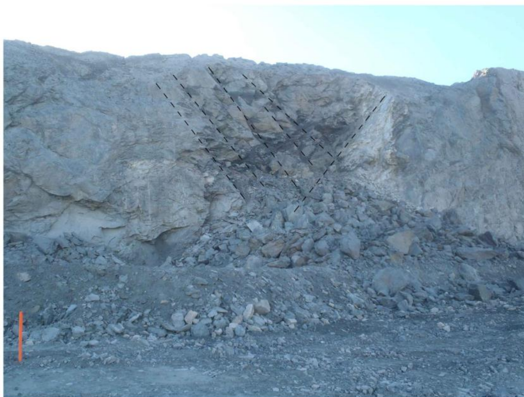
Photograph 4: Overtopping of deflection berm by rock fall on west wall of Pit A on 5109 bench, Stop 2 in Figure 5
