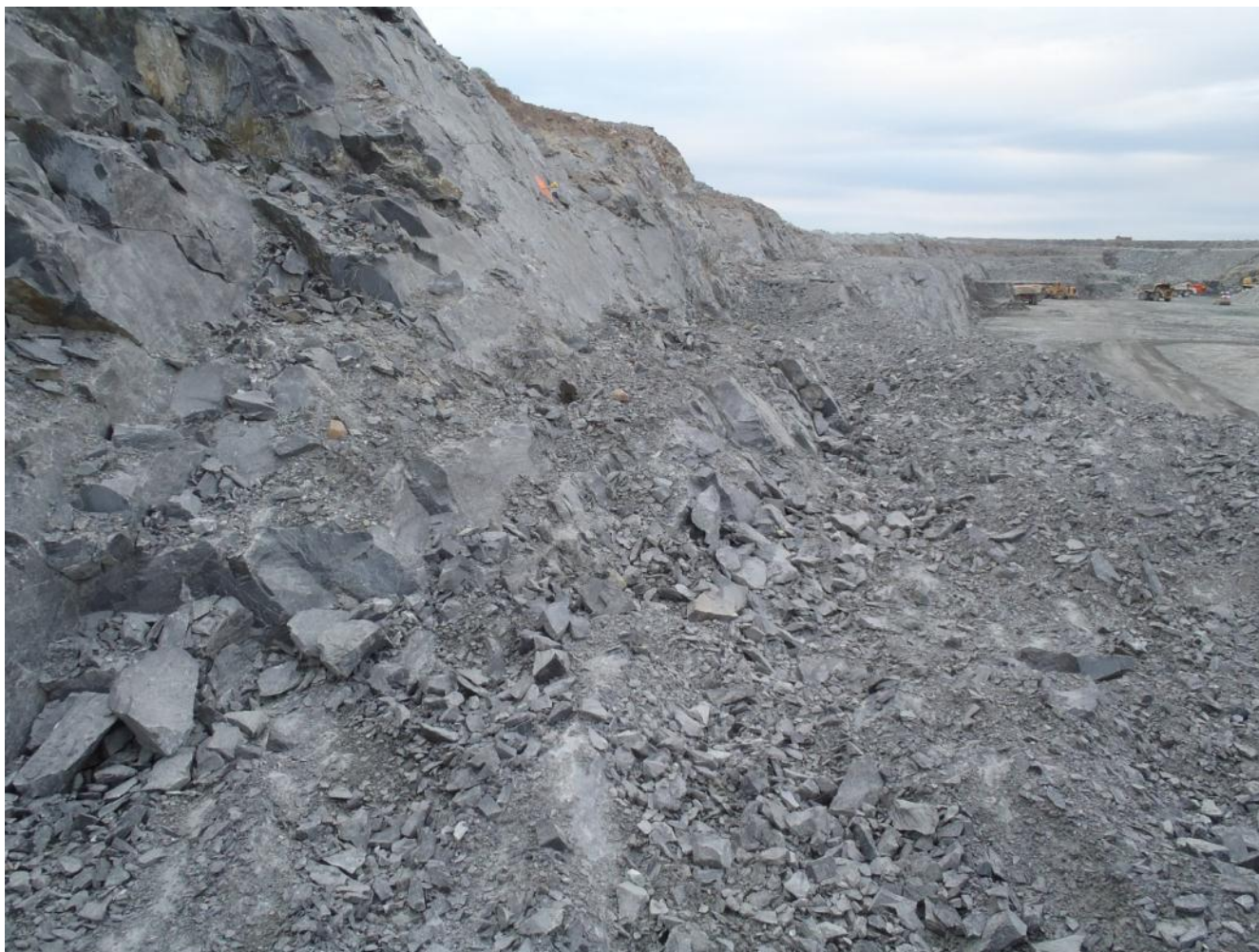
Photograph 34: Shallow dipping foliation at north end of Goose Pit
