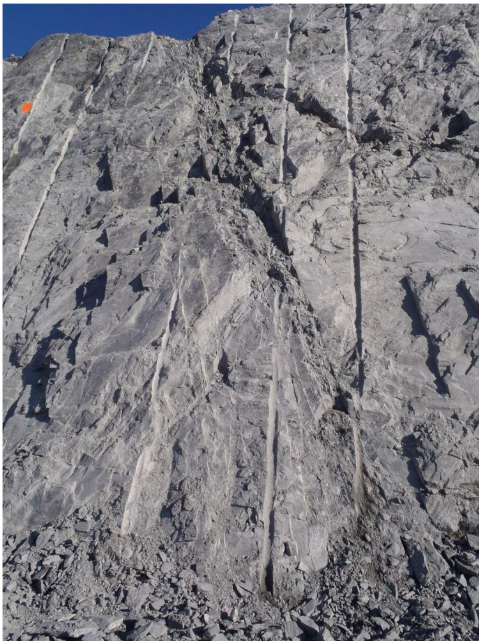
Photograph 32: Discrete fault structure (south dipping) exposed in east wall of Goose Pit
