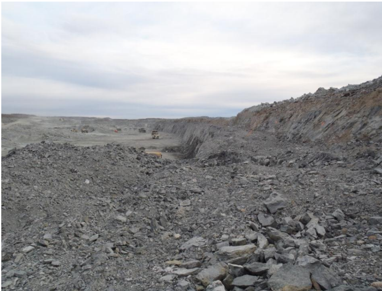
Photograph 35: The 5130 bench of the Goose Pit, showing hummocky appearance and poor cleaning in areas
