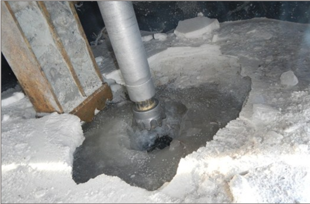
Photo 3: Ice (~12 cm thick) located at BH-11.
