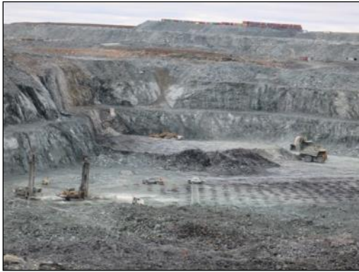
Photo 6: Drills, loaders and shovel in the South Portage pit (also identified as pit E), with drill hole pattern visible in front.
