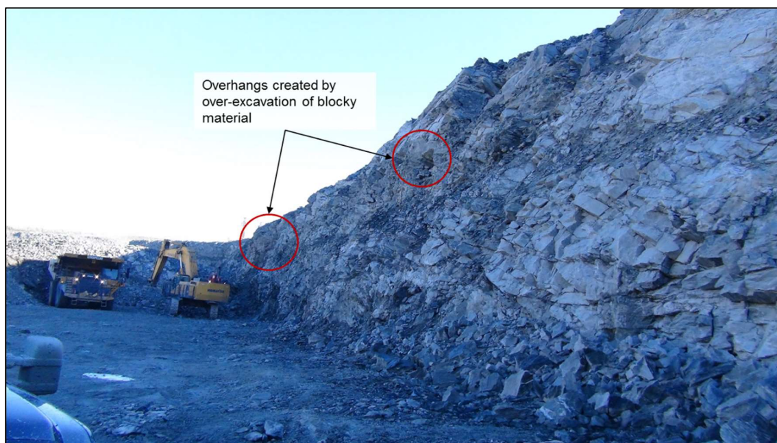
Photograph 8-10: Vault Pit Phase 1 east wall overhangs
