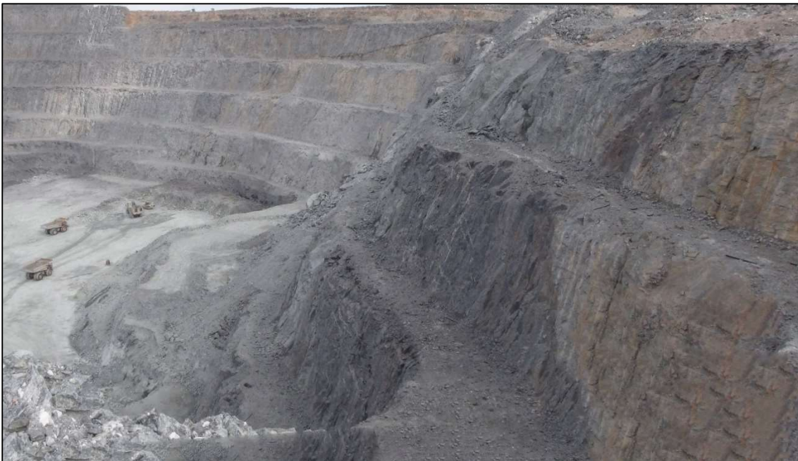
Photograph 6-15: Pit E3 pushback east wall showing local planar failure along continuous north dipping surfaces
