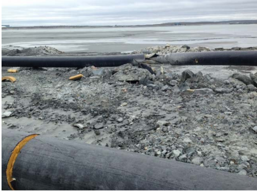
Photo 1 – Pipe damage after the removal of insulation cover
