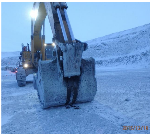
Photo 1 – Hydraulic Oil Spill from Backhoe #11, Vault Pit, December 18 th 2015,
