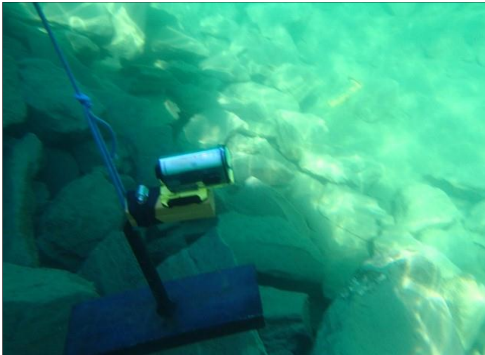
Underwater Video Camera being deployed along Dike face
