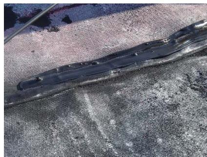
CD-1864 (2018-05-25), looking from Sta. 40+700/-38 m. View of bubbles formed in the extrusion weld because of humidity.
