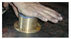
6. Using a slight twisting motion Carefully push Hard Wear Face into Adjuster
