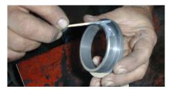
3. Apply epoxy to outer rim of Hard Wear Face (D11)
