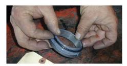
4. Place 'O' Ring (D10) on outer rim of Hard Wear Face (D11). Position 'O' Ring at leading edge.
