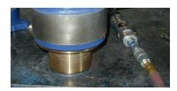
8. Place a heavy object on top of the assembly until dry (min 30 minutes)
