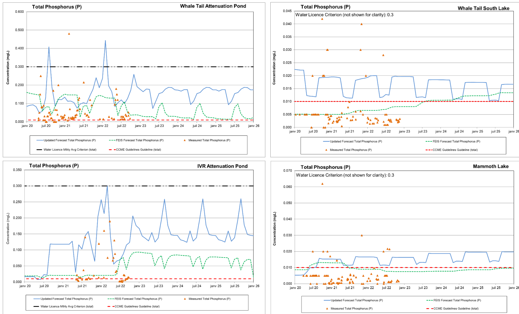
Figure 4-2: Total Phosphorous Forecasted Concentrations during Operation
