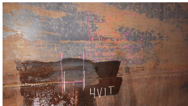
Photo #6: Lack of fusion found T intersection ring level 4 - plate 1 - Top horizontal position
