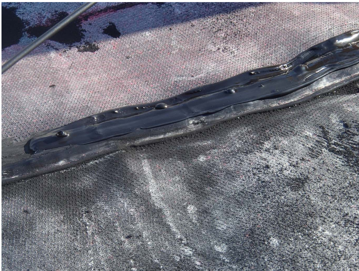
Photograph CD-1864: From Sta. 40+700/-38 m. View of bubbles formed in the extrusion weld because of humidity.
