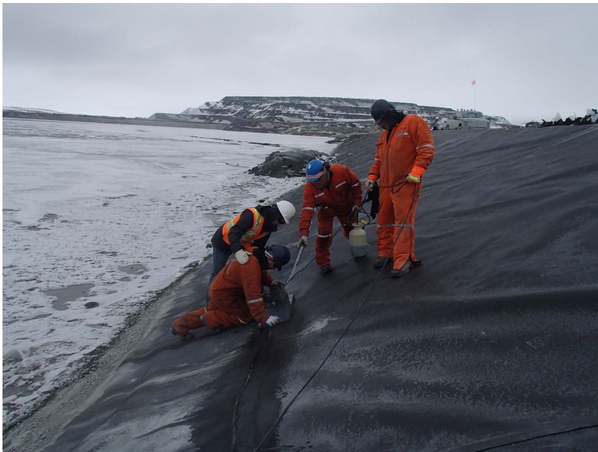
Photograph CD-1875: From Sta. 0+835/-26 m, looking N. View of a vacuum box testing.
