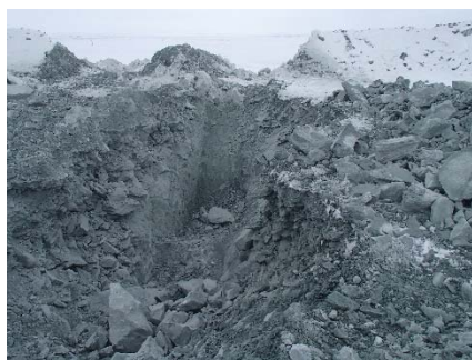
NCIS-001 (2018-05-19). View of a test pit in the UM rockfill lift at El. 152 m: a thick layer of snow (2 m) underlies the rockfill.
