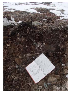
NCIS-015 (2018-05-22), looking S from Sta. 1+850 m. View of the 200 mm deep test pit excavated into the natural soil. A thin layer of organic soil overlies frozen till.
