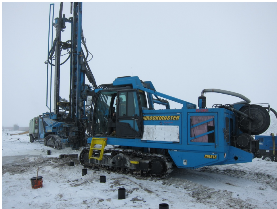
Photograph 91: Rockmaster 100 DTH drill rig for casing installation and triconing - April 1, 2011
