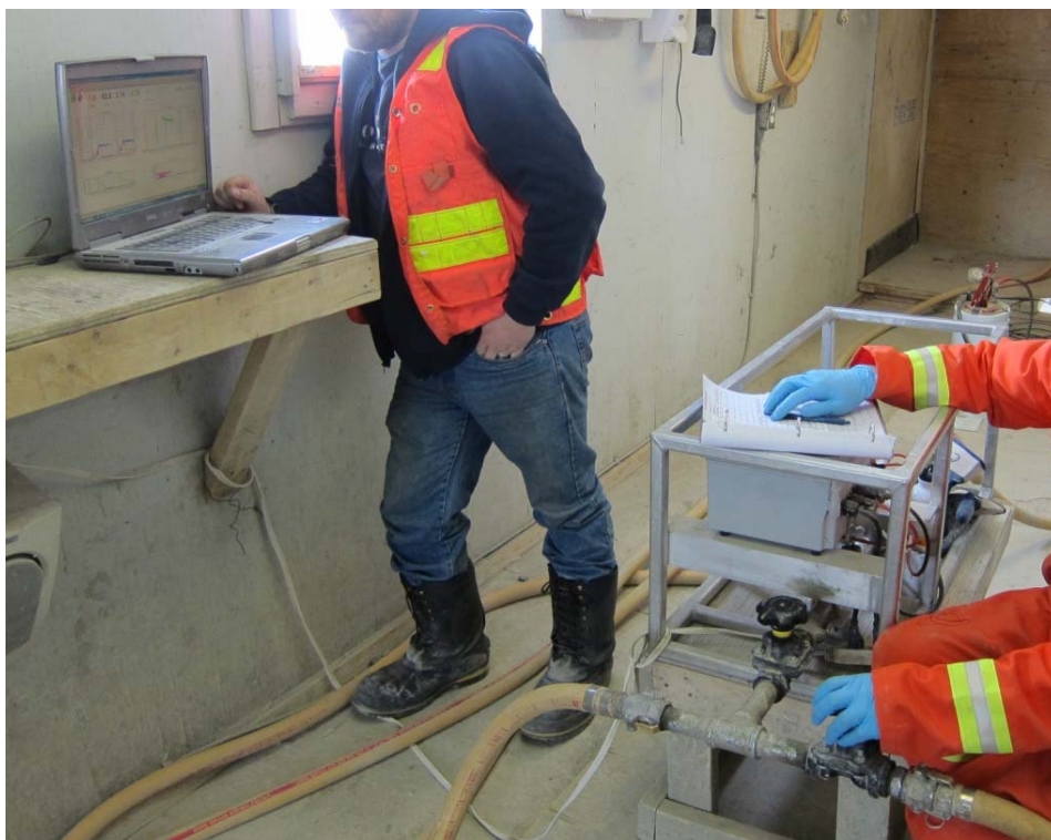
Photograph 95: RST Permeation Grout Monitoring System with field laptop for real-time monitoring - April 15, 2011
