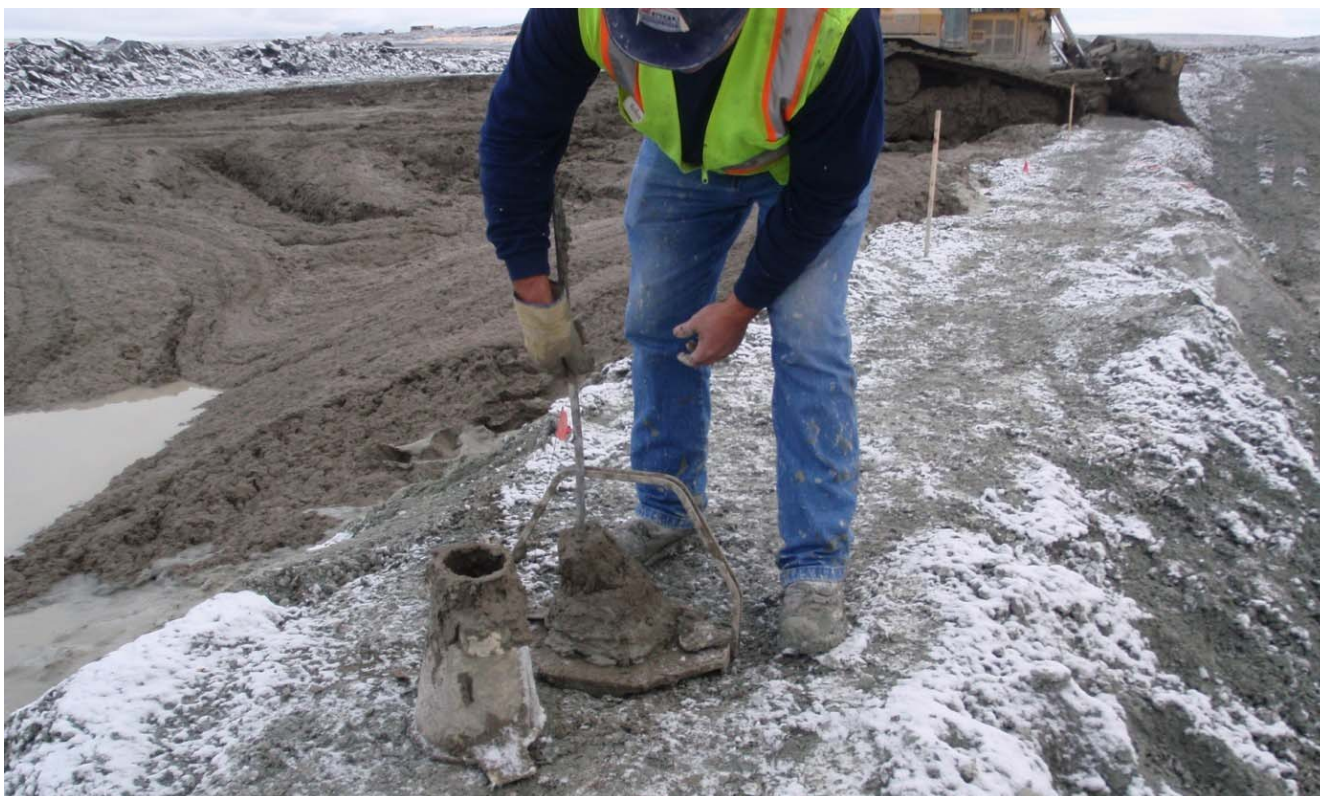
Photograph 33: Slump test carried out on a sample of soil bentonite taken from Sta. 30+455 - September 22, 2009
