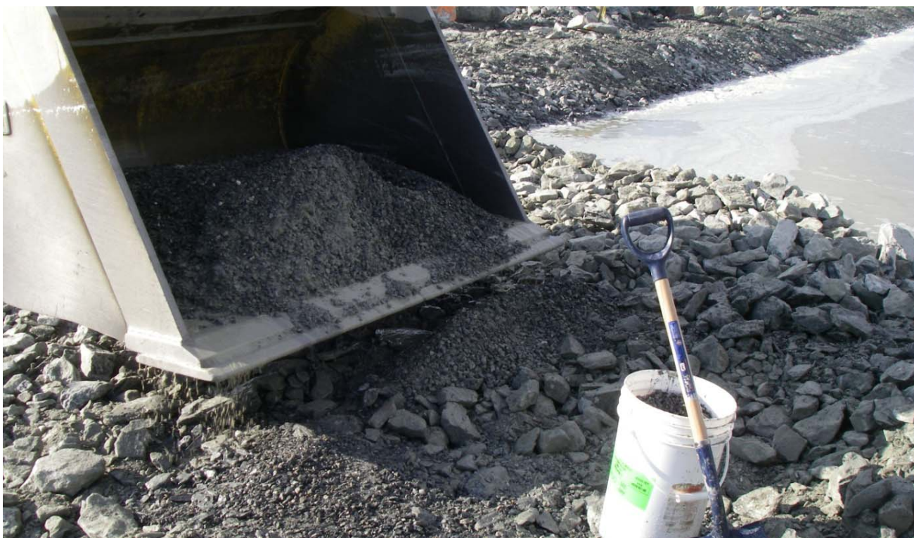
Photograph 16: In-situ sampling of the Core Backfill taken from Sta.30+284 - August 22, 2009
