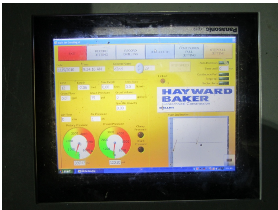
Photograph 108: Jet drilling / grouting monitoring screen - November 5, 2010
