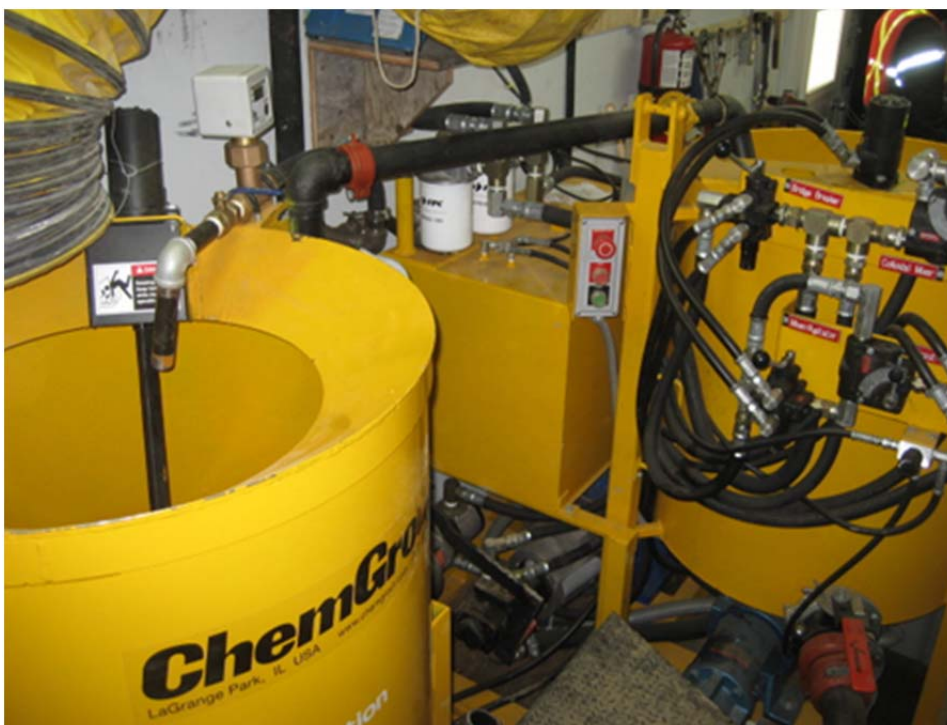
Photograph 94: Chemgrout CG-680 3L8_EH High Shear Colloidal Mixer/Agitator with Moyno Pump - October 11, 2008
