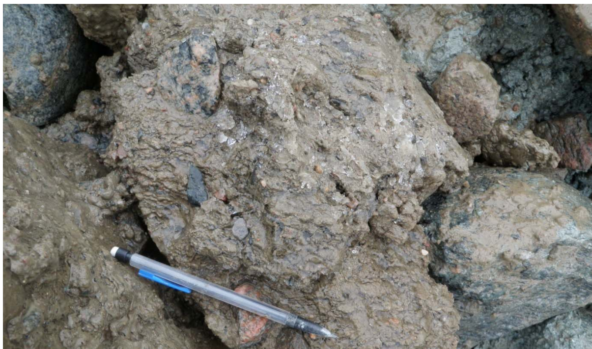
Photograph 63: Sample of ice-rich till excavated at Sta. 32+127 - September 14, 2010
