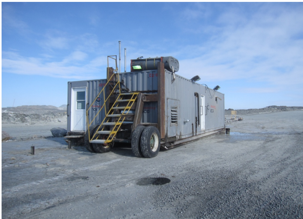
Photograph 89: All-weather, mobile grouting plant - April 2010
