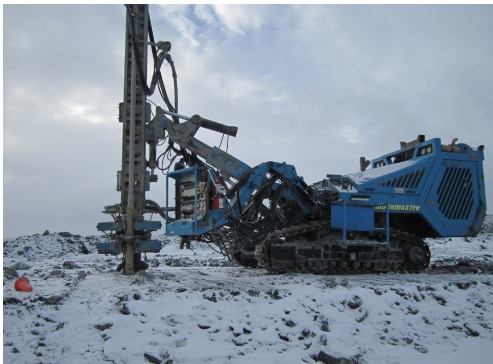
Photograph 92: Rockmaster 80 DTH drill rig for casing installation and triconing - October 13, 2010
