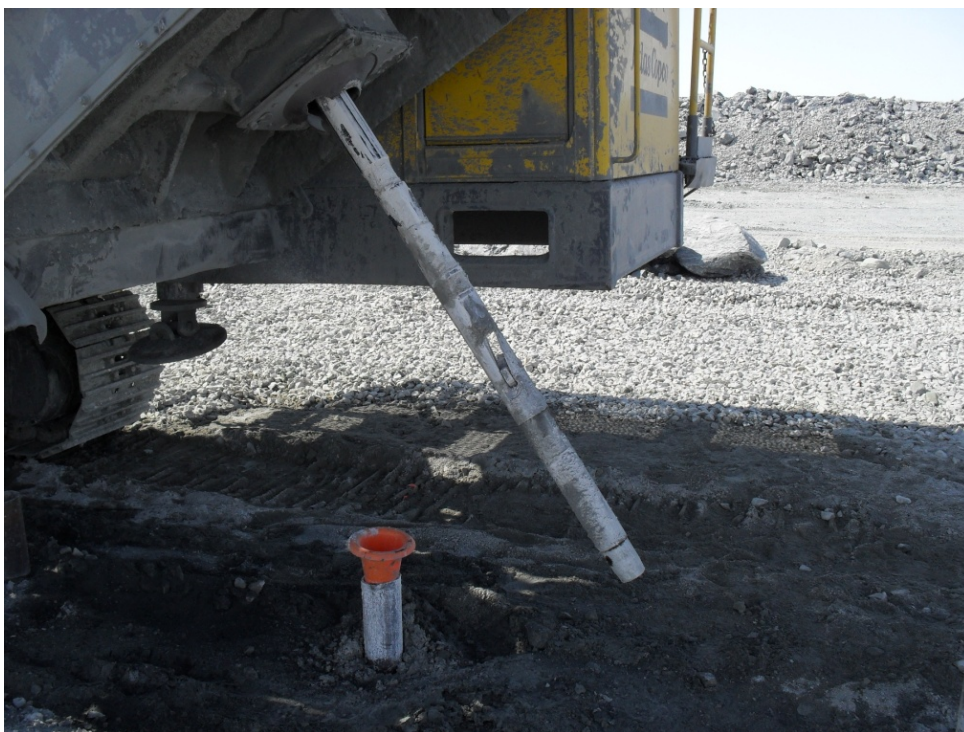
Photograph 97: Holte steel casing perforator tool - June 4, 2010
