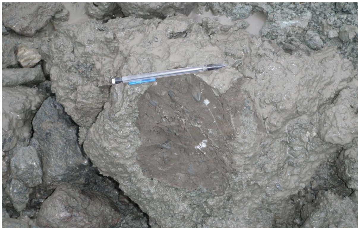
Photograph 62: Sample of competent till excavated at Sta. 32+062 - September 11, 2010
