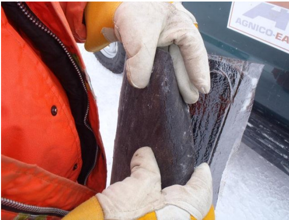
(Mar 1 2013) Cracks in Teranap geomembrane from bending it with hands
