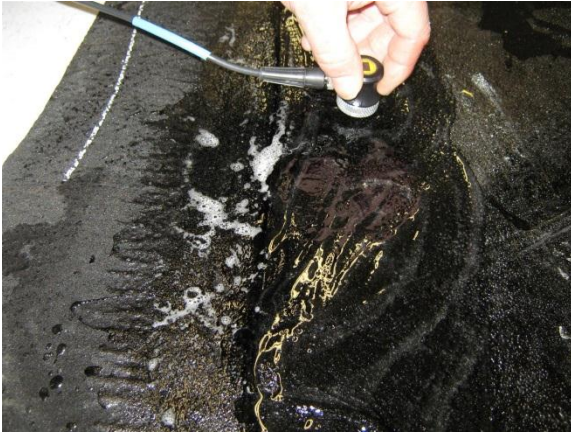
(Mar 1 2013) Testing the Teranap geomembrane for permeability
