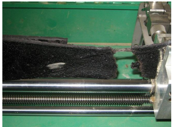
(Mar 1 2013) Stretch testing the Teranap geomembrane
