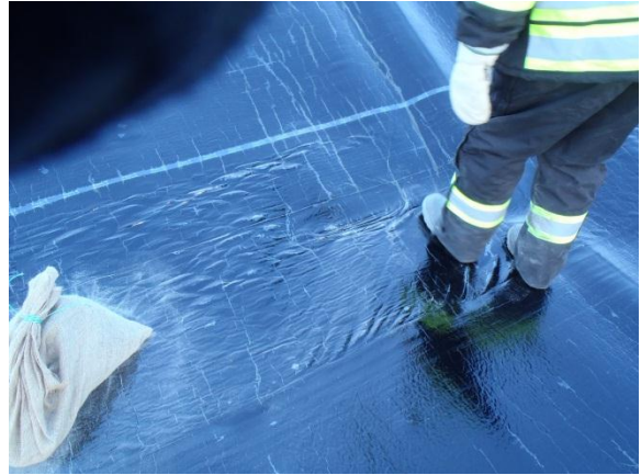
(Feb 28 2013) Cracks in geomembrane created by stepping on it
