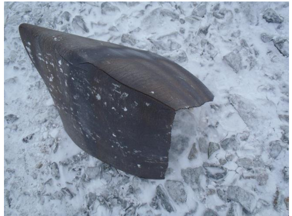
(Mar 1 2013) Rip in Teranap geomembrane from running over it with a truck
