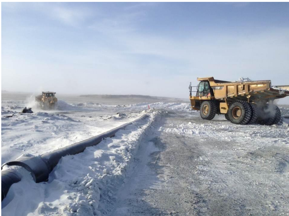
Figure 2.2: CAT D8T clearing snow from drill pattern
