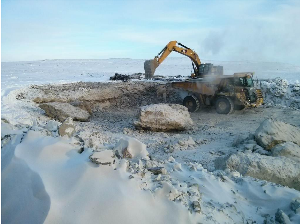
Figure 2.5: CAT 345D loading a CAT 773F haul truck behind a few till boulders
