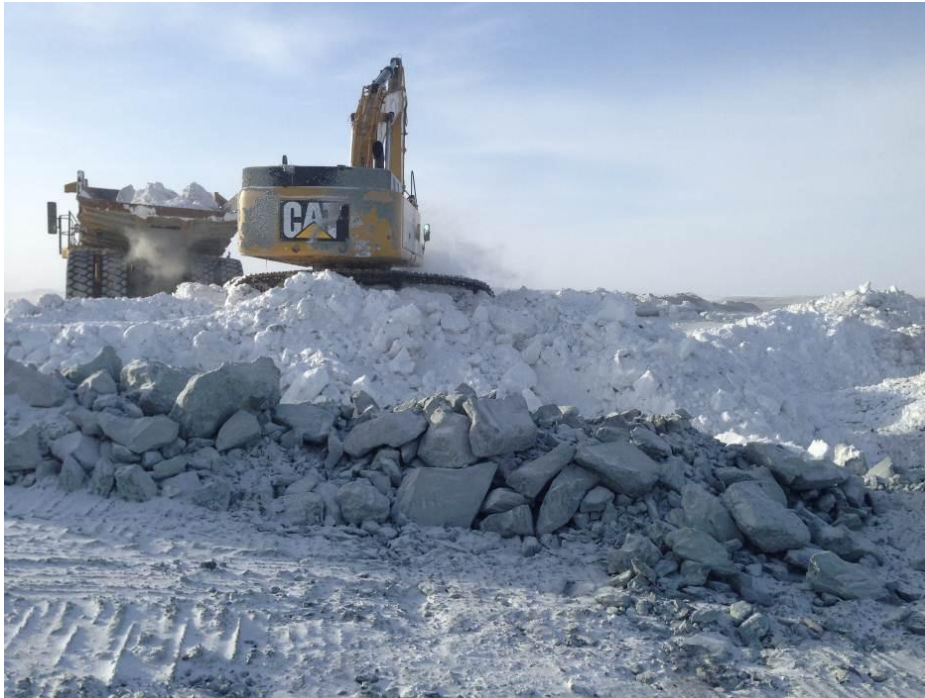
Figure 2.1: CAT 345D loading a CAT 773F haul truck with snow
