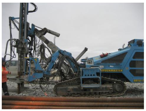
Photograph 67: Rockmaster 990 DTH Drill Rig for Casing Installation – September 26, 2008.
