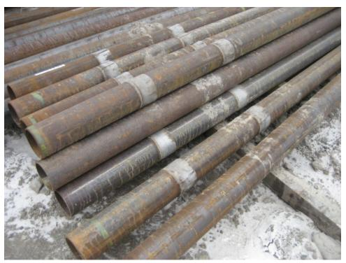
Photograph 69: Modified Casing with Injection Ports - September 26, 2008
