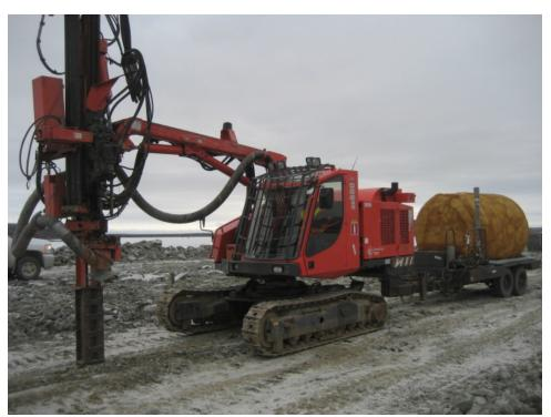
Photograph 73: Tamrock 996 Top Hammer Drill Rig for Bedrock Drilling – October 16, 2008
