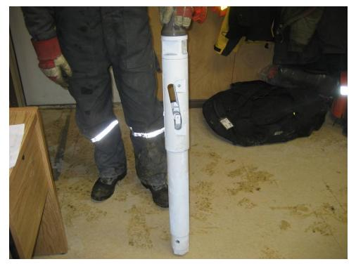
Photograph 75: Holte Perforator Tool – January 19, 2009
