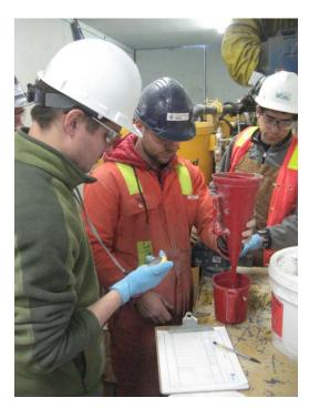
Photograph 88: Quality Assurance of Mix Viscosity Measuring Marsh Funnel Time - November 11, 2008
