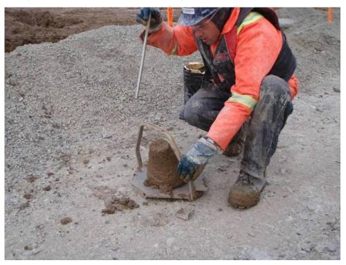
Photograph 45: A QC sump test result of 75 mm for the SB backfill conducted by FGL at Sta. 60+391, September 16, 2008.
