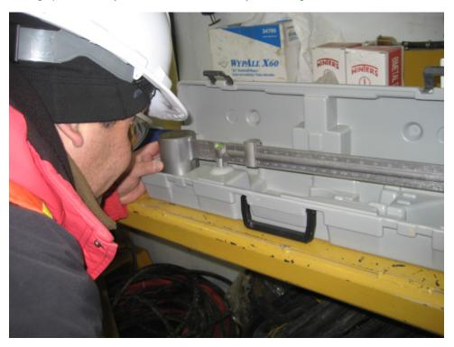
Photograph 89: Quality Assurance Measuring Specific Gravity of Grout Mix using Mud Balance – October 12, 2008
