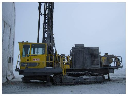
Photograph 74: Atlas Copco DM45 Drill Rig for Perforating – February 17, 2009
