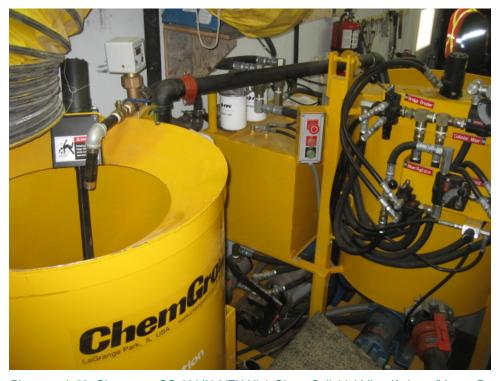
Photograph 82: Chemgrout CG-680/3L8/EH High Shear Colloidal Mixer/Agitator/Moyno Pump – October 11, 2008
