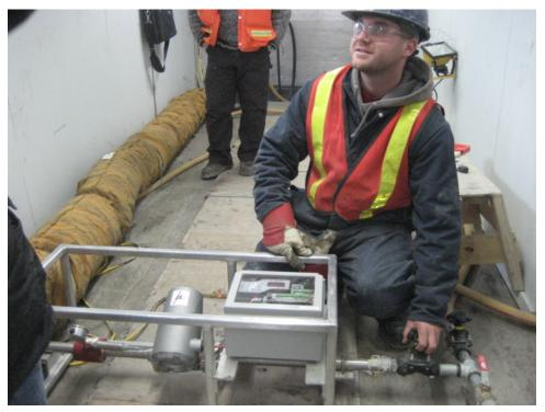
Photograph 84: RST Permeation Grout Monitoring System – November 5, 2008
