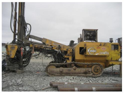
Photograph 68: Rockmaster 945 DTH Drill Rig for Casing Installation – September 26, 2008.
