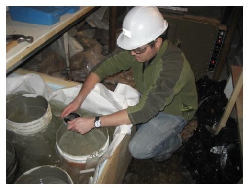
Photograph 91: Grout Mix Design Measuring Set Time Using Pilcon Hand Vane - November 11, 2008
