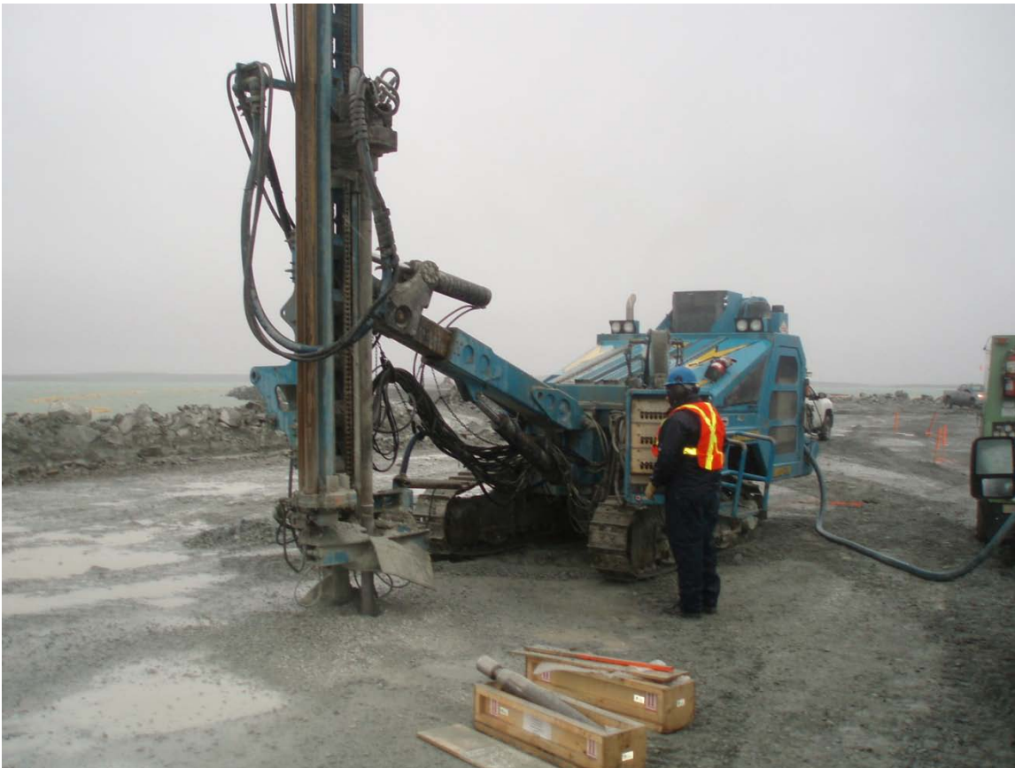
Photograph 4: Rockmaster RM-115 ITH air rotary pneumatic, downhole hammer drill rig
