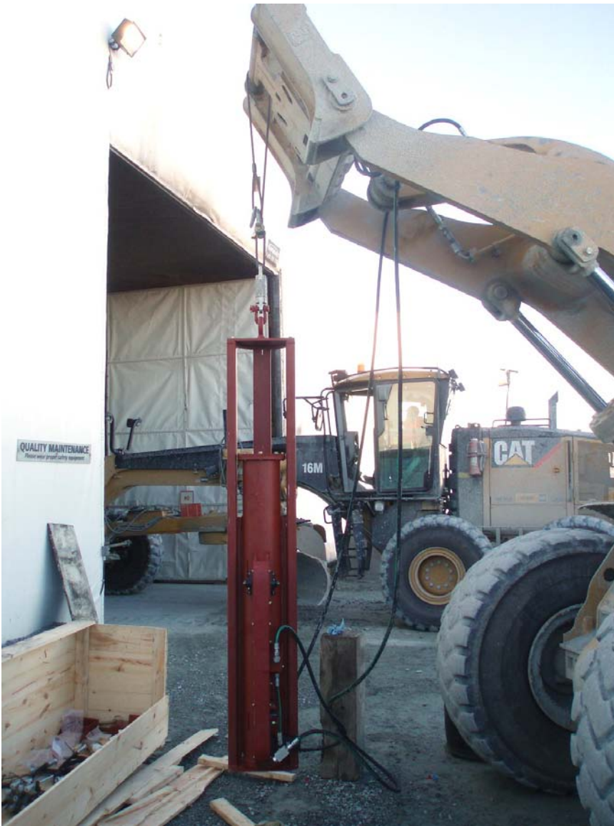
Photograph 5: Caterpillar 966 Loader with LPT hammer attached
