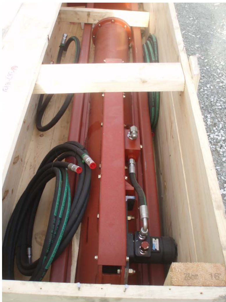
Photograph 2: Foremost-Mobile 109.1 kg (240 lbs.) self-compensating, automatic drop hammer
