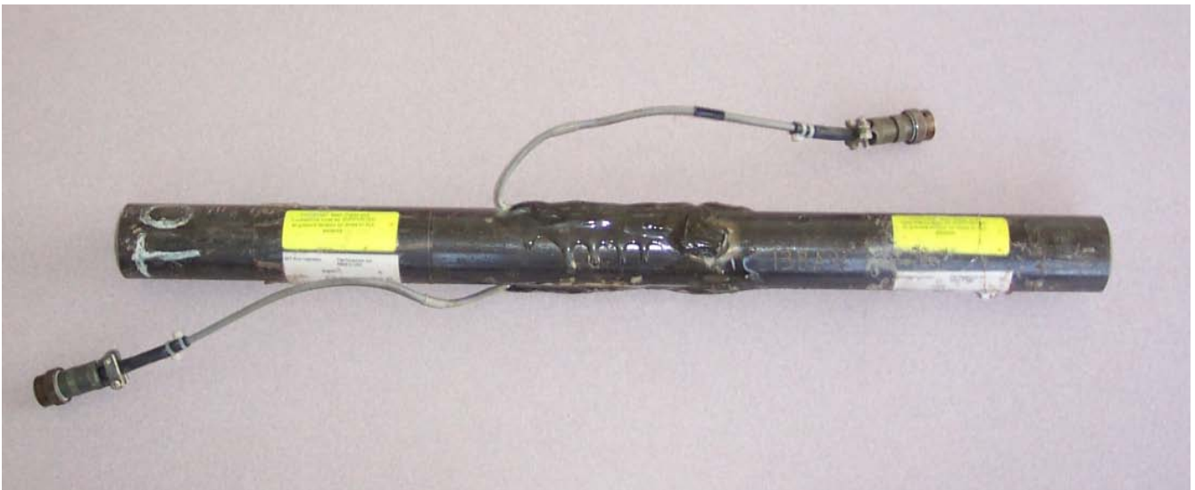
Photograph 3: Pile Driver Analyzer. NW drill rod fixed with two strain gauges and two accelerometers
