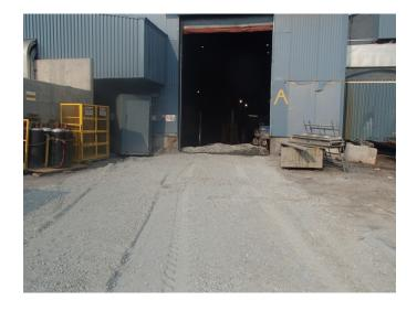
Spill area mixed with rock material to absorb
