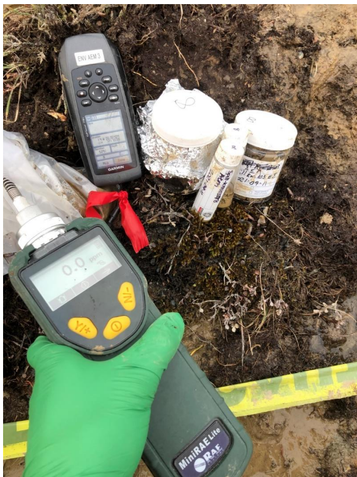
Figure 7. Use of PID and soil sampling following excavation (2021-09-11)
