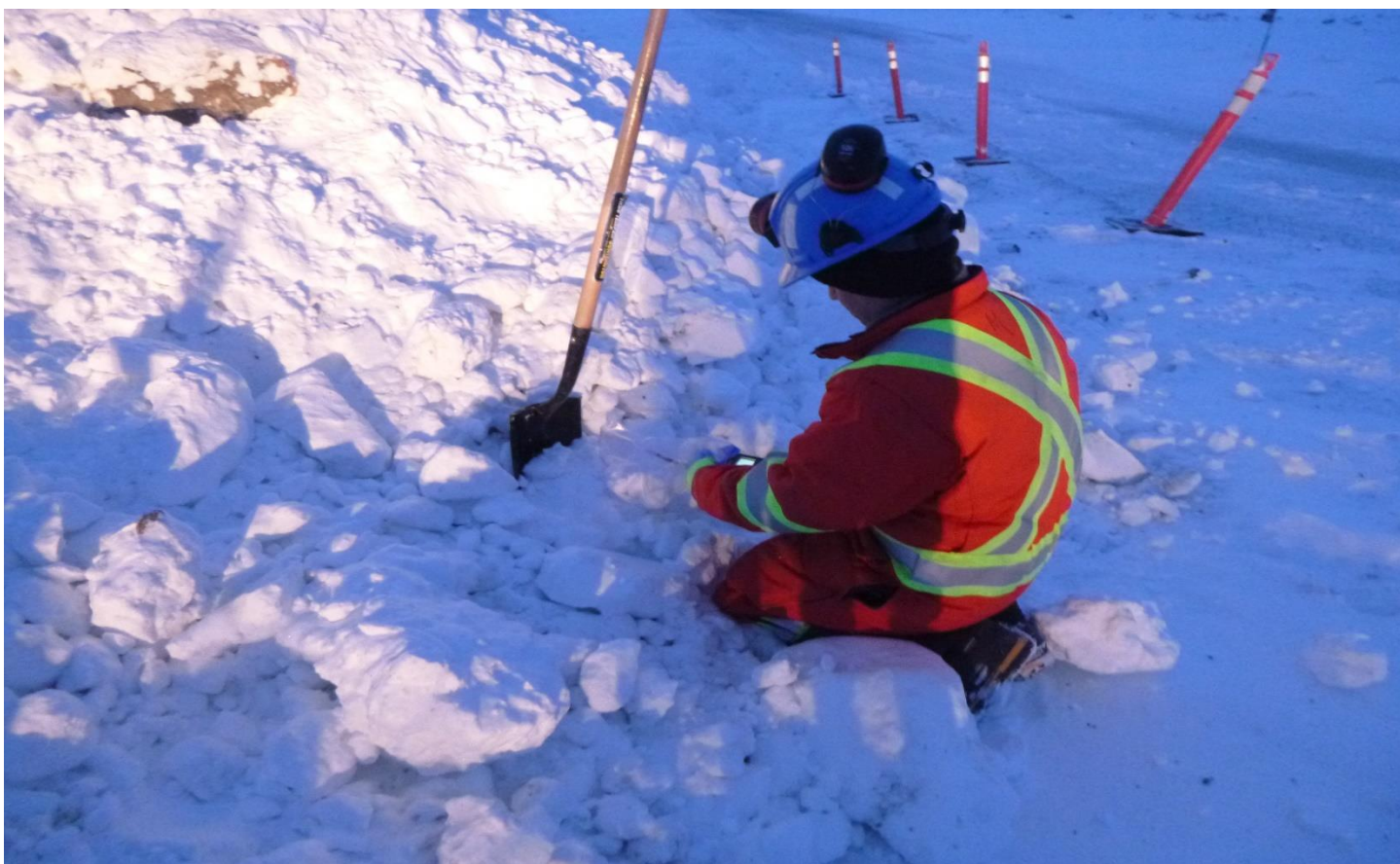
Figure 12. Snow testing with PID after removal - 2022-12-06
