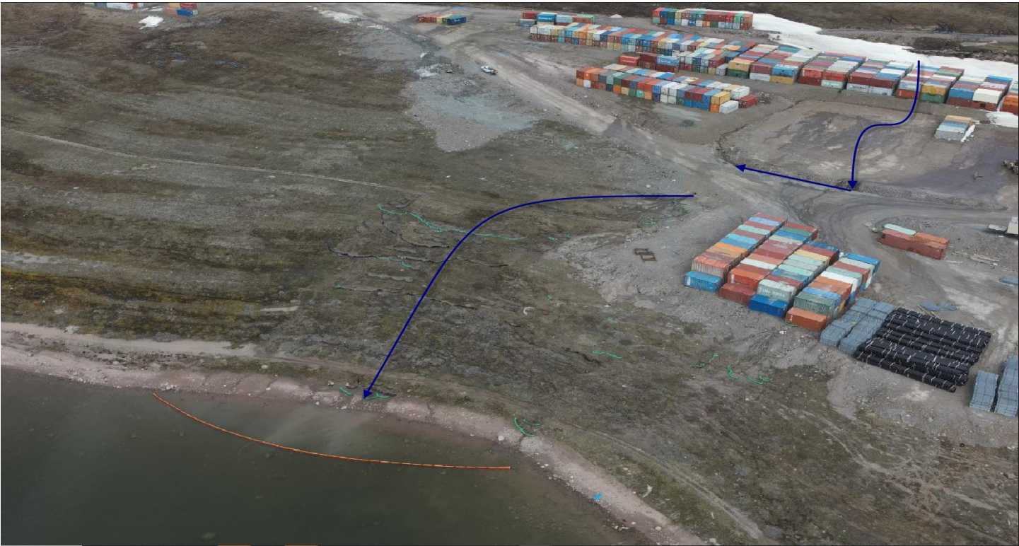
Figure 2. Aerial view of Baker Lake shore after Agnico Eagle’s intervention and deployment of turbidity control measures showing the new flow path
