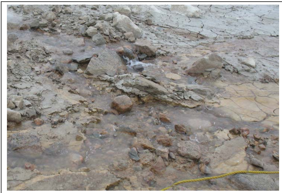
Photo # 6 East Dike, seepage to west of ramp, note slightly cloudy
