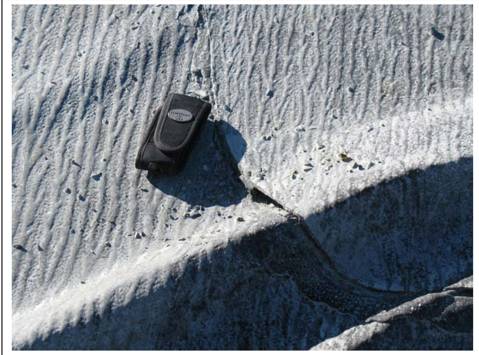
Photo # 13 Stormwater dike, liner weld failure at wrinkle
