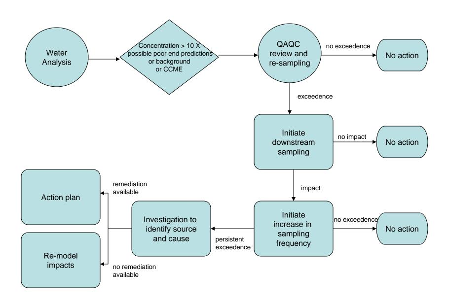
Figure 3-2: Logic Diagram for Non-Regulated Discharge
