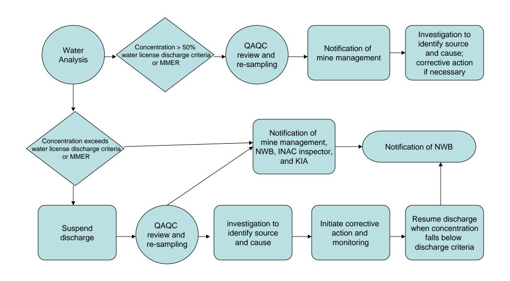
Figure 3-1: Logic Diagram for Regulated Discharge
