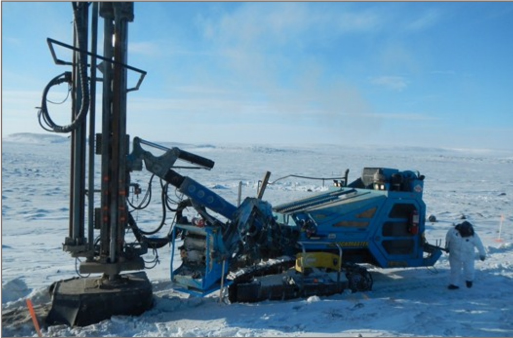
Photo 1: Southwest view of the down hole air hammer drill drilling BH-18.
