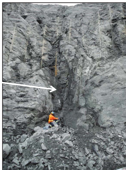
July - Sampling groundwater on Pit A north wall, not enough water was flowing to sample this wall seepage in September
