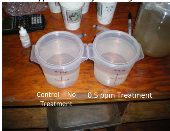
Figure 4.1-1. Comparing no Treatment vs. 0.5 ppm Chitosan After Settling 20 hrs
