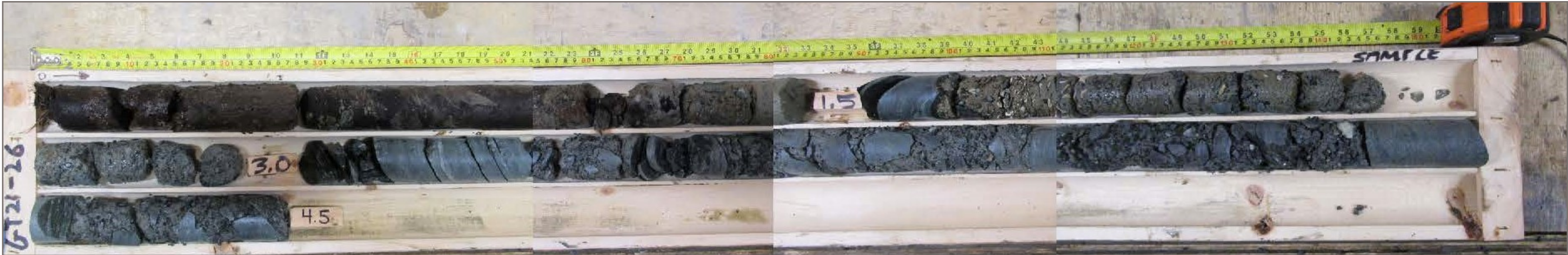
Photo 63: GT21-26 overburden core; depth 0.0 – 4.5 m
