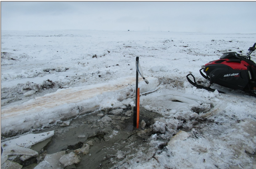
Photo 59: GT21-20 multi-bead GTC installation; depth 15.0 m
