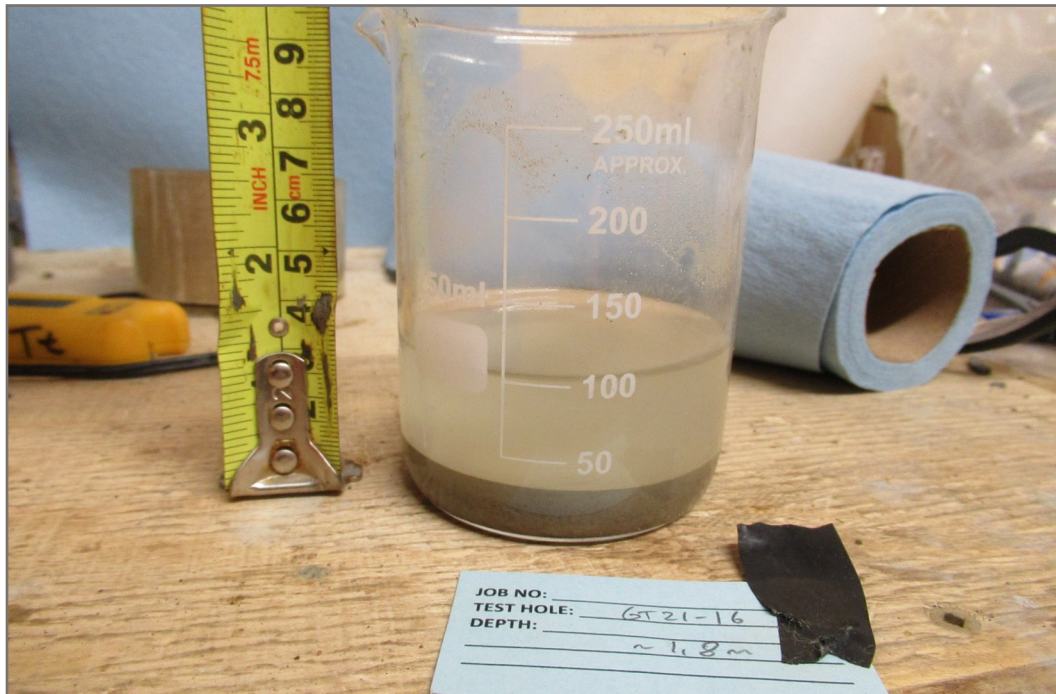
Photo 31: GT21-16 jar test; depth 1.8 m
