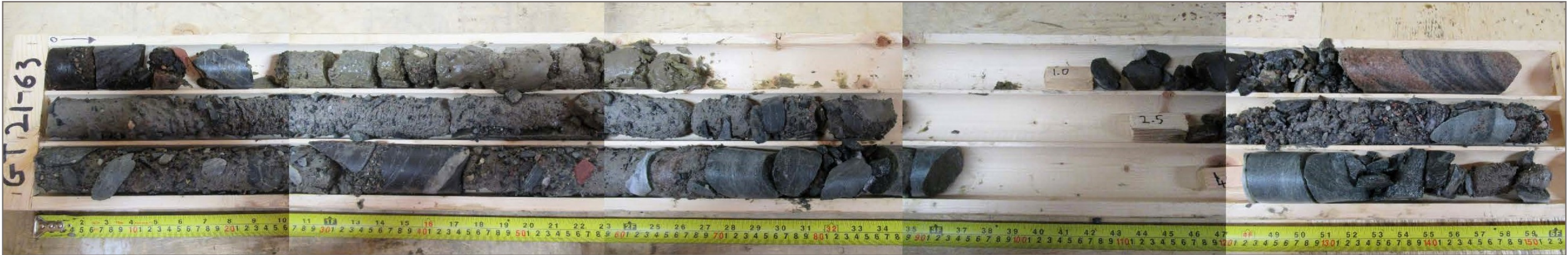
Photo 74: GT21-63 overburden core; depth 0.0 – 4.3 m
