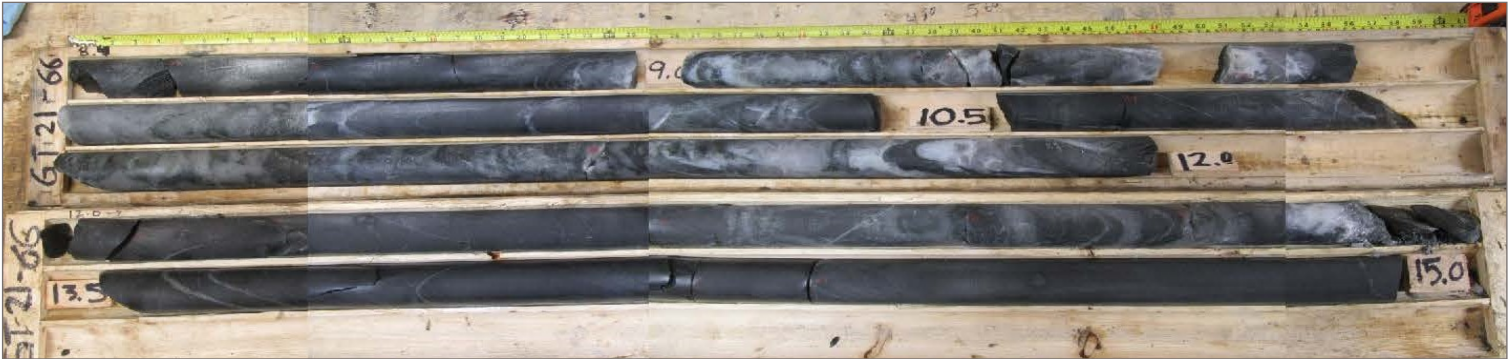
Photo 102: GT21-66 bedrock core; depth 8.4 – 15.0 m
