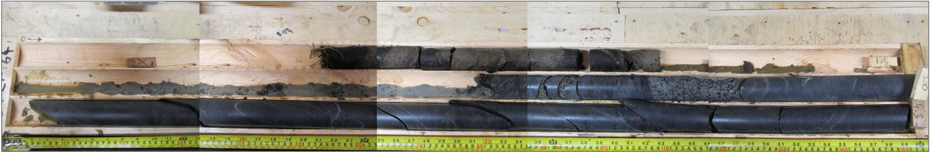
Photo 93: GT21-64 bedrock core; depth 3.0 – 4.5 m
