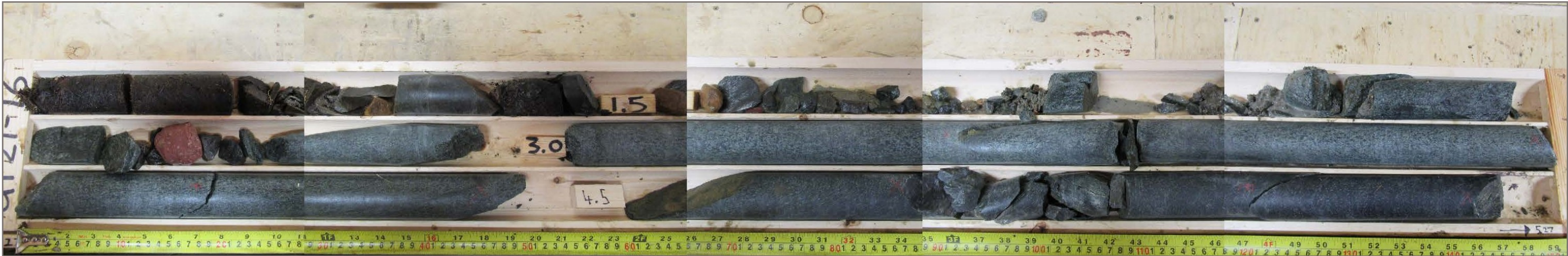
Photo 27: GT21-16 overburden & bedrock core; depth 2.5 – 5.27 m
