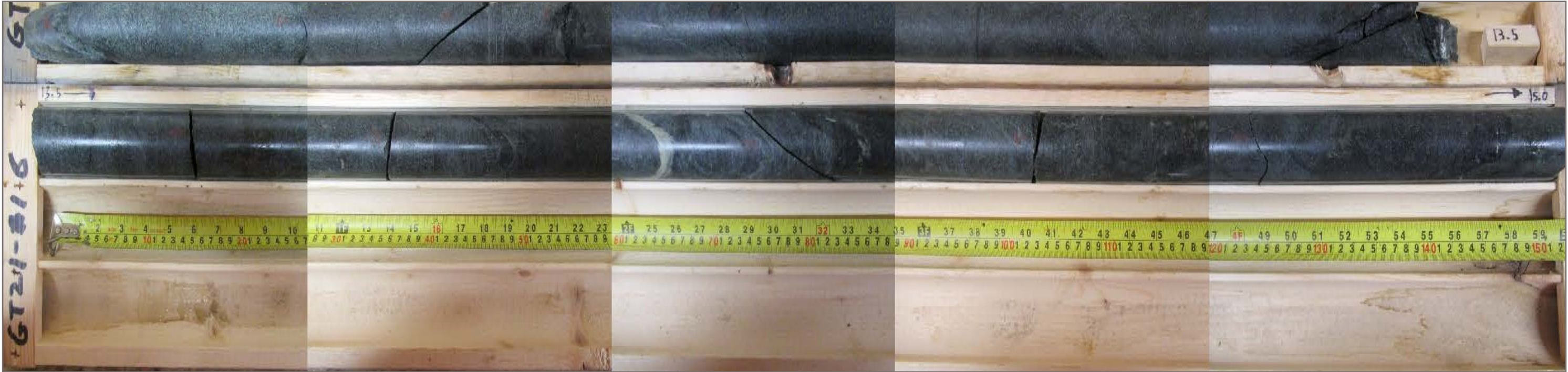
Photo 30: GT21-16 bedrock core; depth 13.5 – 15.0 m
