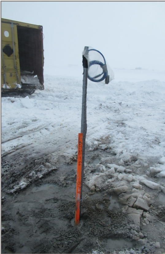
Photo 103: GT21-66 multi-bead GTC installation; depth 14.15 m
