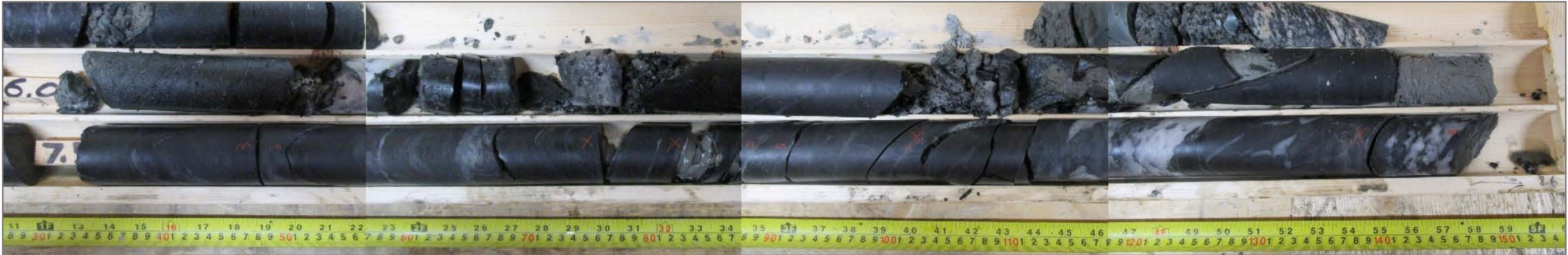
Photo 70: GT21-45 bedrock core; depth 7.5 – 8.6 m
