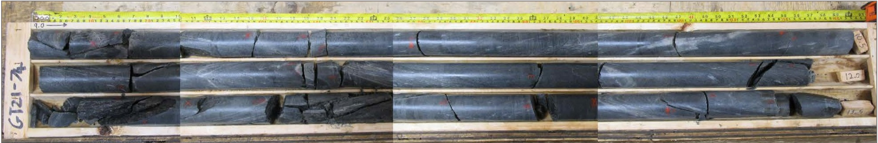
Photo 88: GT21-74 bedrock core; depth 9.0 – 13.5 m
