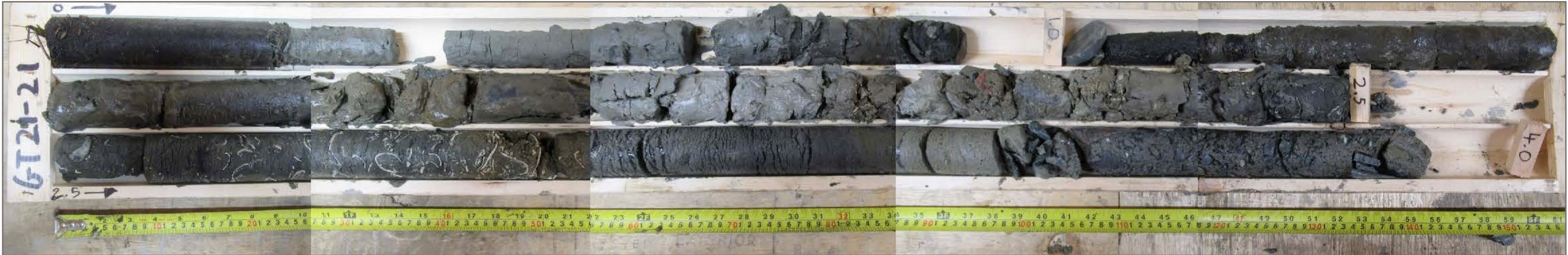
Photo 60: GT21-21 overburden core; depth 0.0 – 4.0 m
