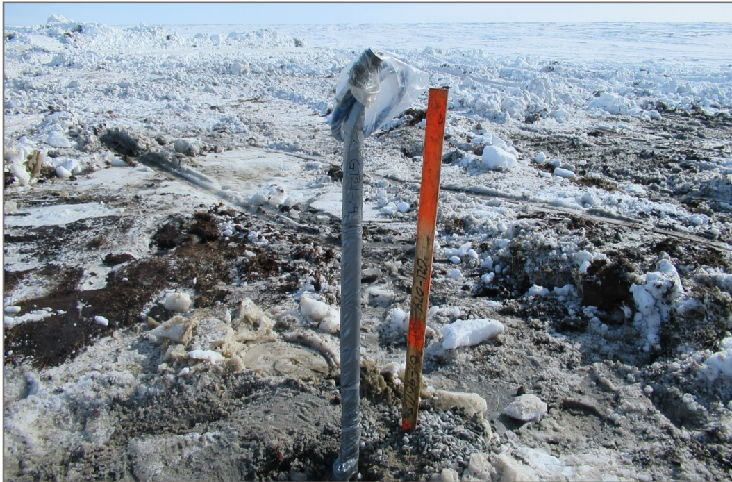
Photo 91: GT21-74 multi-bead GTC installation; depth 14.4 m
