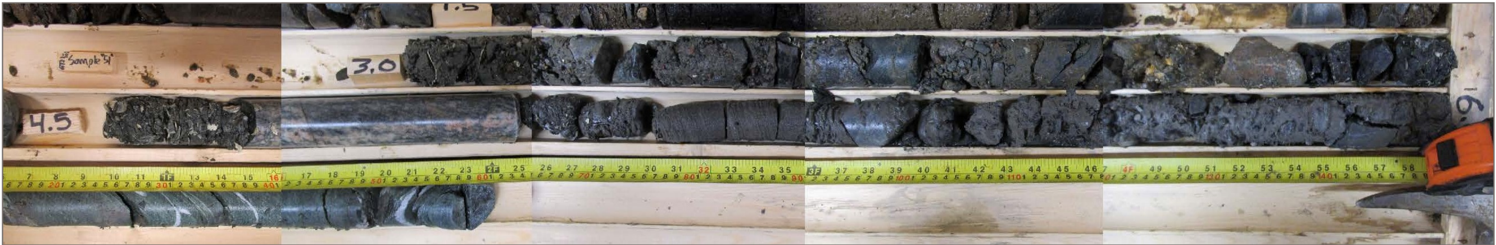
Photo 111: GT21-102 overburden core; depth 4.5 – 6.0 m
