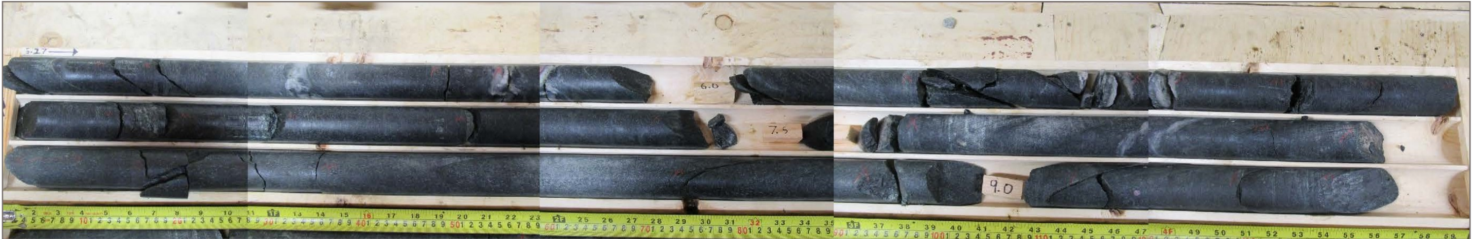
Photo 28: GT21-16 bedrock core; depth 5.27 – 9.3 m
