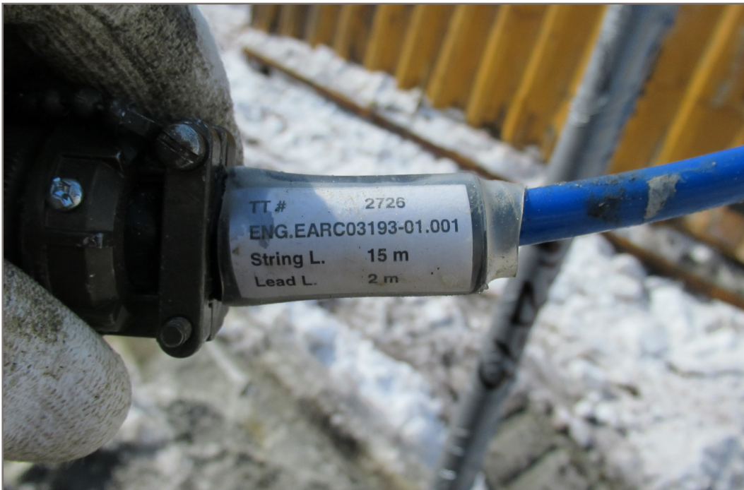
Photo 85: GT21-73 multi-bead GTC installation; depth 15.0 m
