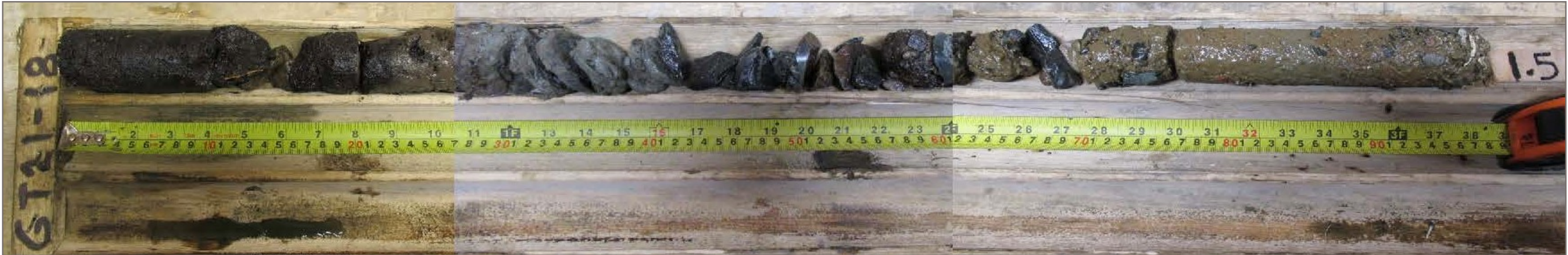
Photo 40: GT21-18 overburden core; depth 0.0 – 1.5 m
