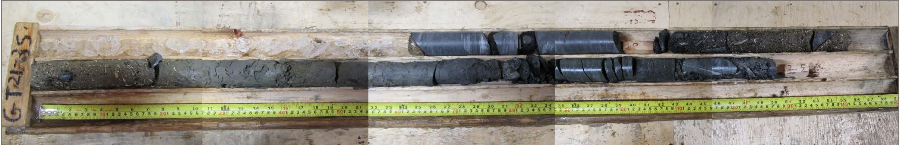
Photo 1: GT21-60 (35) overburden core; depth 0.0 – 2.5 m
