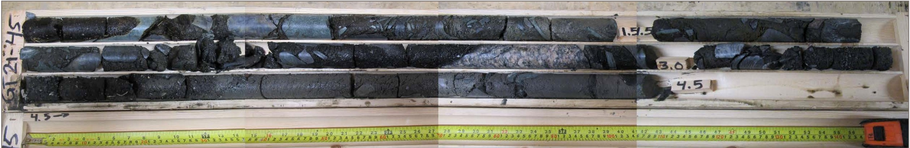
Photo 68: GT21-45 overburden core; depth 0.0 – 4.5 m
