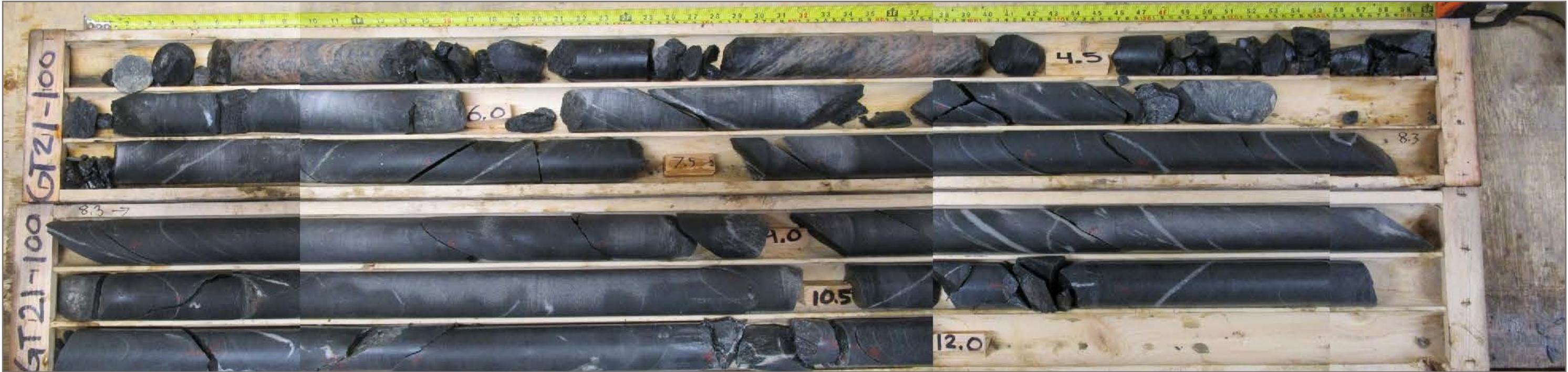
Photo 107: GT21-100 overburden & bedrock core; depth 0.0 – 12.0 m
