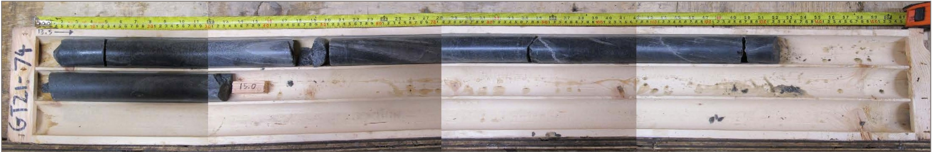
Photo 89: GT21-74 bedrock core; depth 13.5 – 15.0 m
