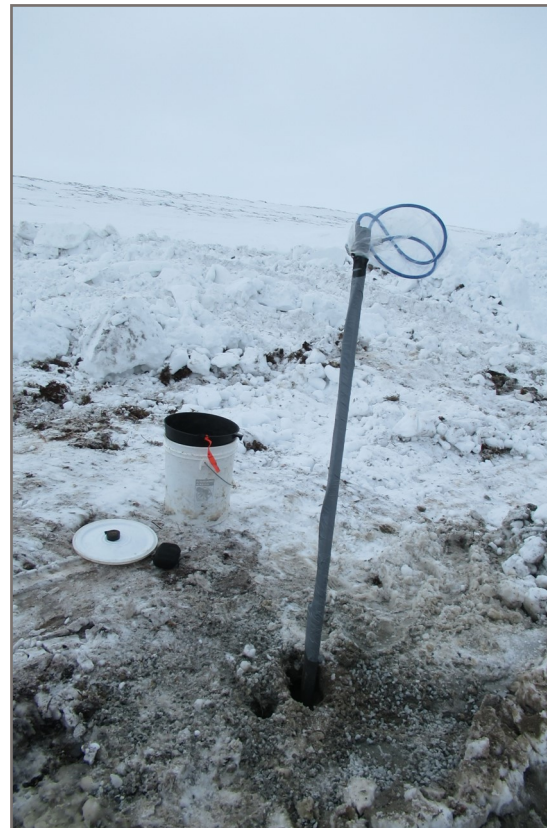
Photo 115: GT21-102 multi-bead GTC installation; depth 14.4 m
