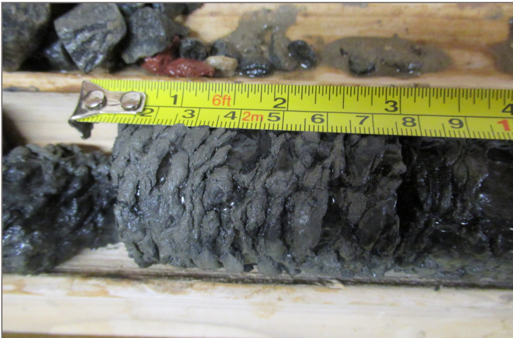
Photo 10: GT21-61 (36) overburden core; depth 2.5 m
