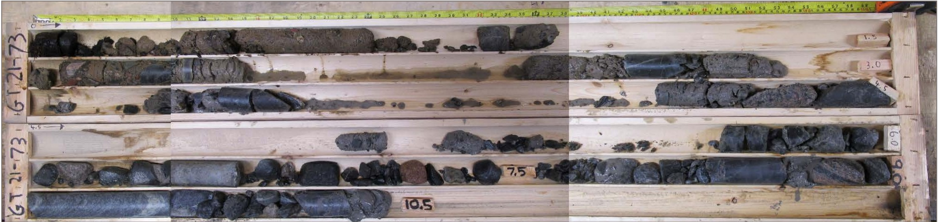
Photo 81: GT21-73 overburden core; depth 6.0 – 10.5 m
