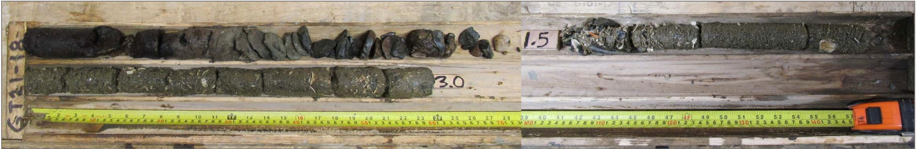
Photo 41: GT21-18 overburden core; depth 1.5 – 3.0 m
