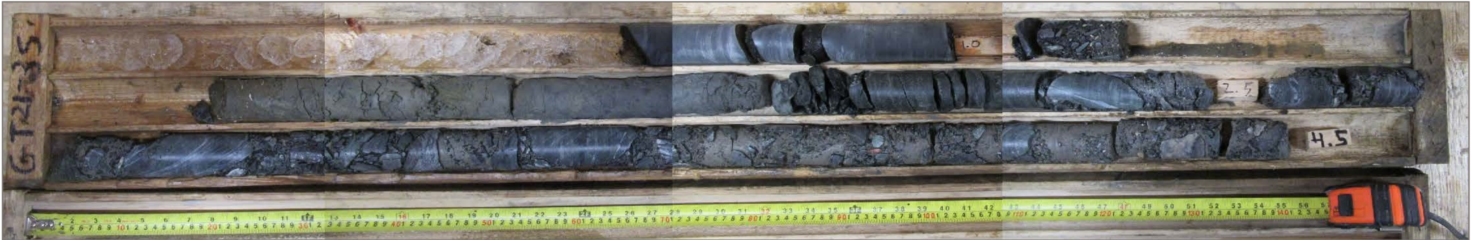
Photo 2: GT21-60 (35) overburden core; depth 2.5 – 4.5 m
