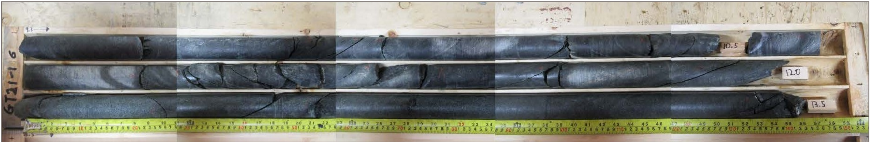
Photo 29: GT21-16 bedrock core; depth 9.3 – 13.5 m
