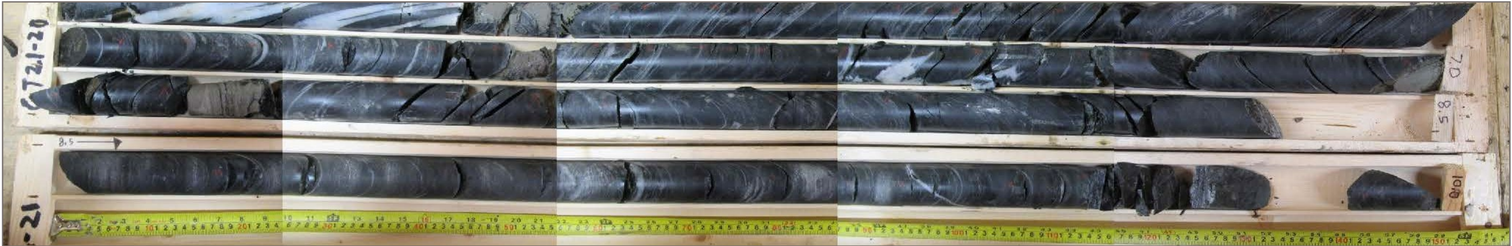
Photo 61: GT21-21 bedrock core; depth 4.0 – 10.0 m
