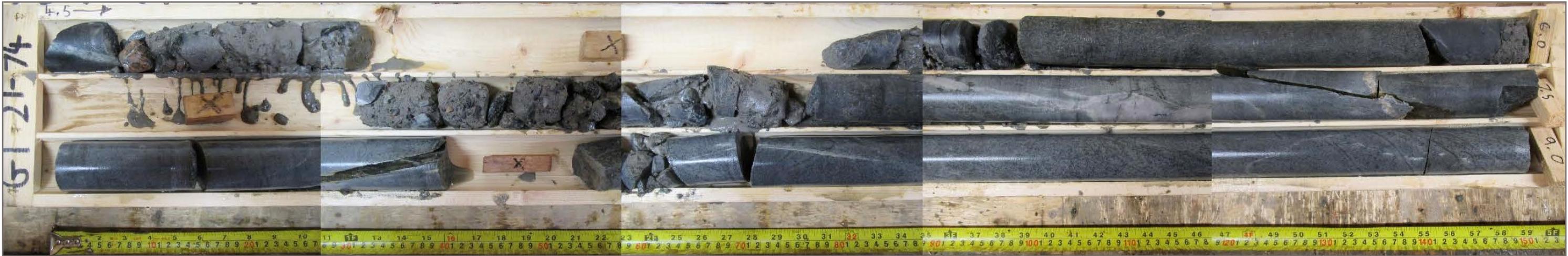
Photo 87: GT21-74 overburden & bedrock core; depth 4.5 – 9.0 m
