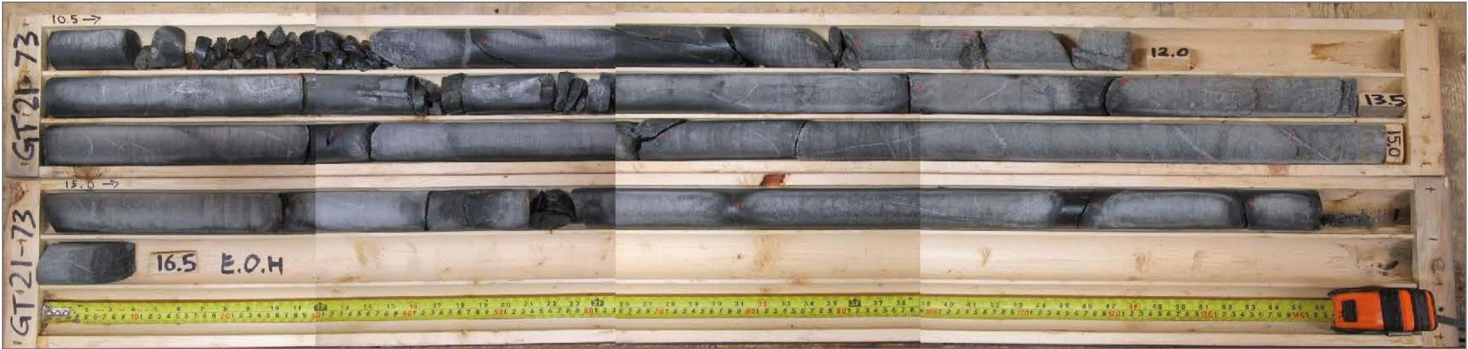
Photo 82: GT21-73 bedrock core; depth 10.5 – 16.5 m
