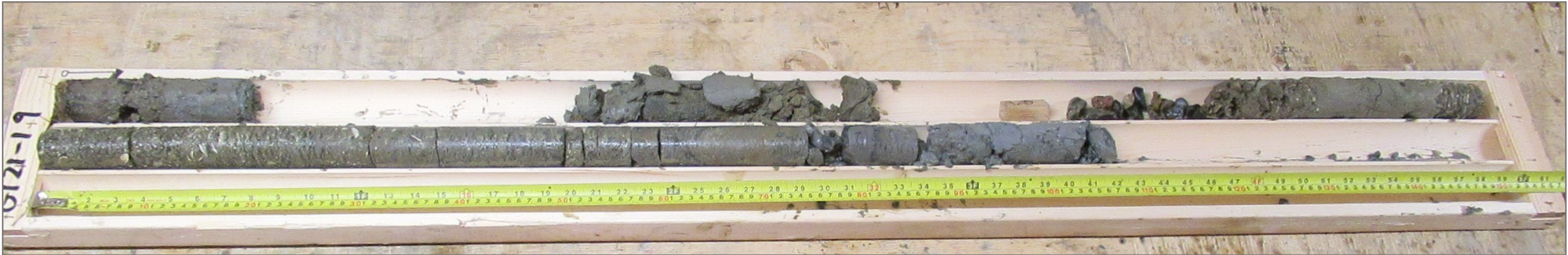
Photo 48: GT21-19 overburden core; depth 1.0 – 2.5 m
