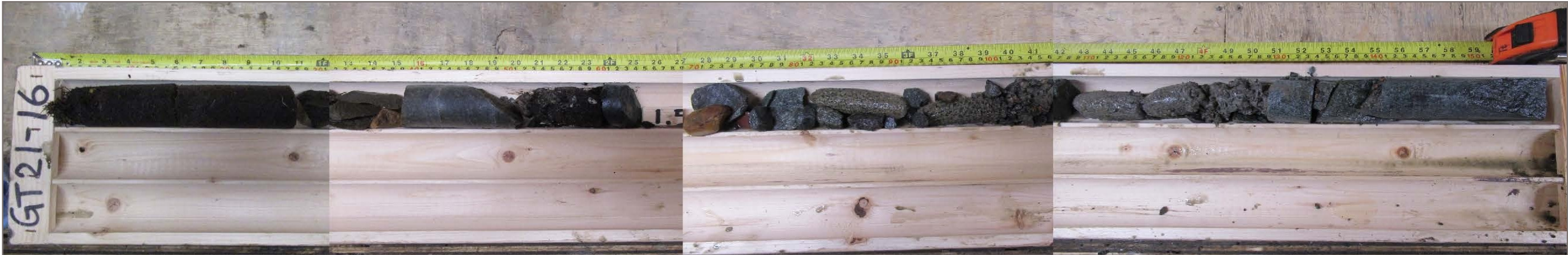
Photo 26: GT21-16 overburden core; depth 0.0 – 2.5 m
