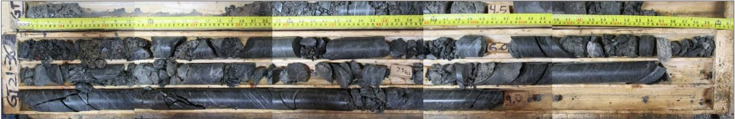
Photo 13: GT21-61 (36) overburden core; depth 7.5 – 9.0 m
