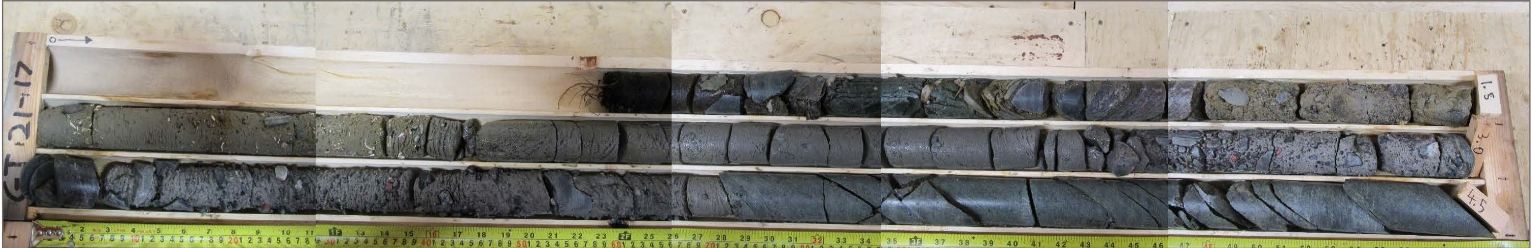
Photo 34: GT21-17 overburden core; depth 0.0 – 4.5 m
