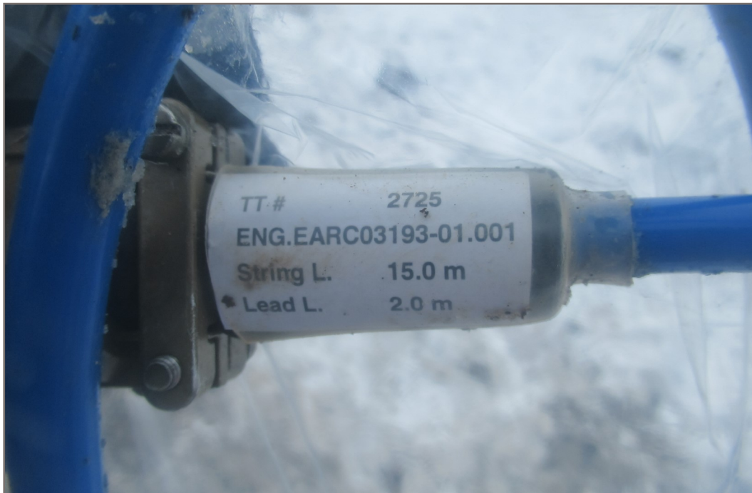
Photo 116: GT21-102 multi-bead GTC installation; depth 14.4 m
