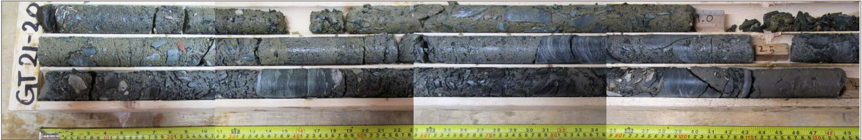
Photo 53: GT21-20 overburden & bedrock core; depth 0.0 – 4.14 m
