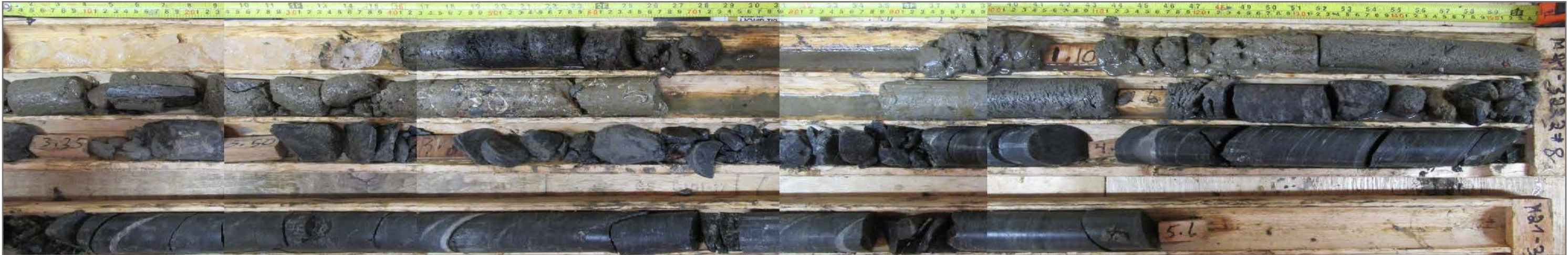
Photo 22: GT21-62 (37) overburden & bedrock core; depth 3.35 – 5.6 m
