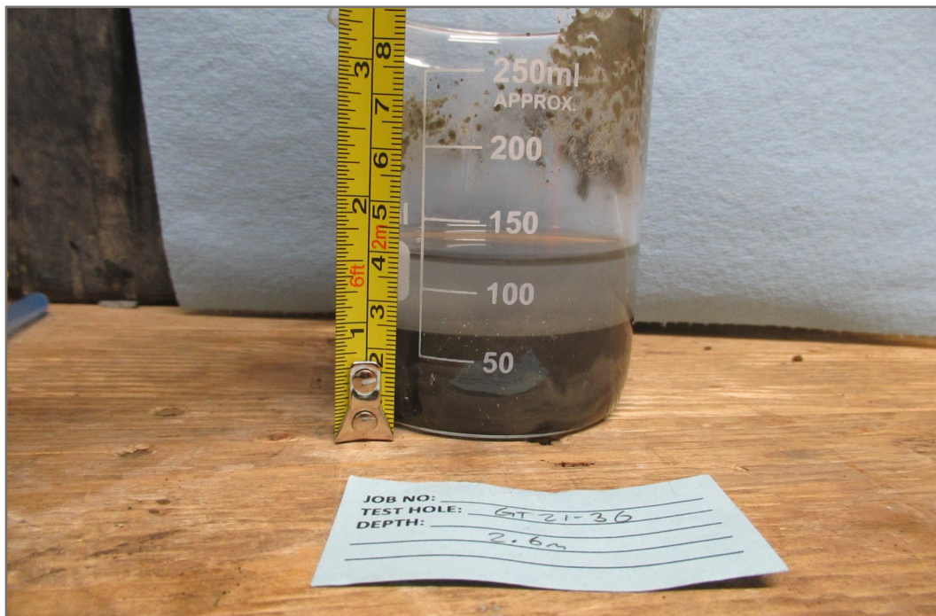
Photo 17: GT21-61 (36) jar test; depth 2.6 m
