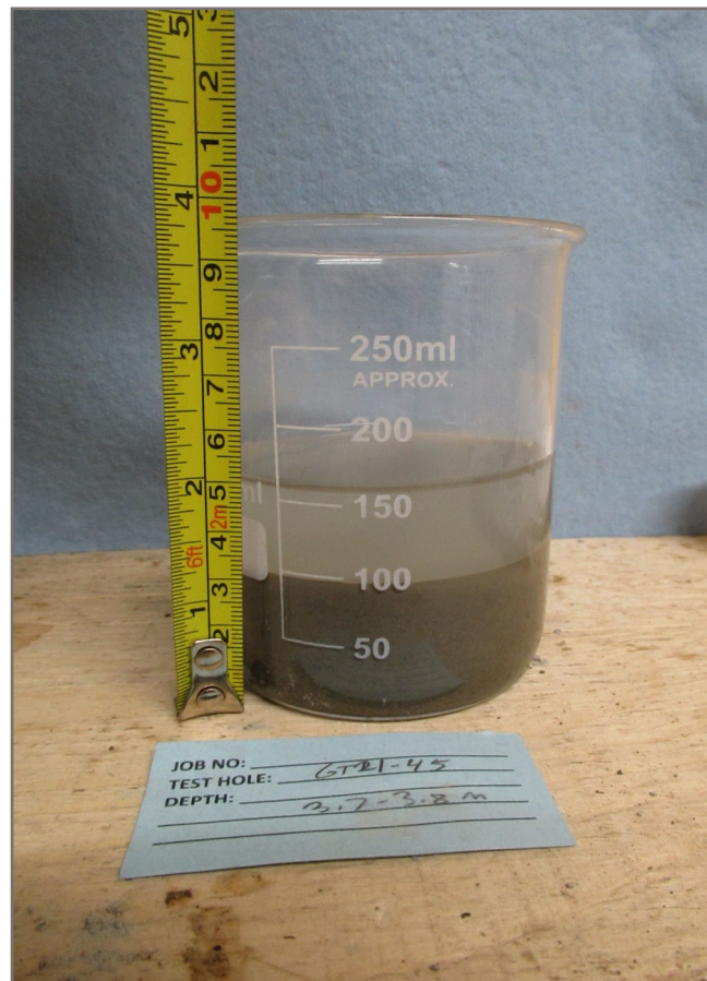
Photo 73: Photo 73 – GT21-45 jar test; depth 3.7 – 3.8 m
