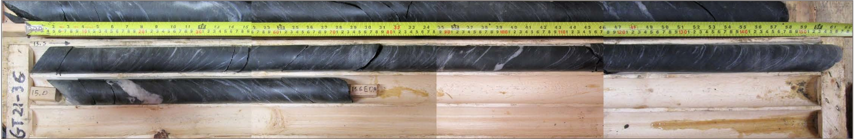
Photo 15: GT21-61 (36) bedrock core; depth 13.5 – 15.6 m
