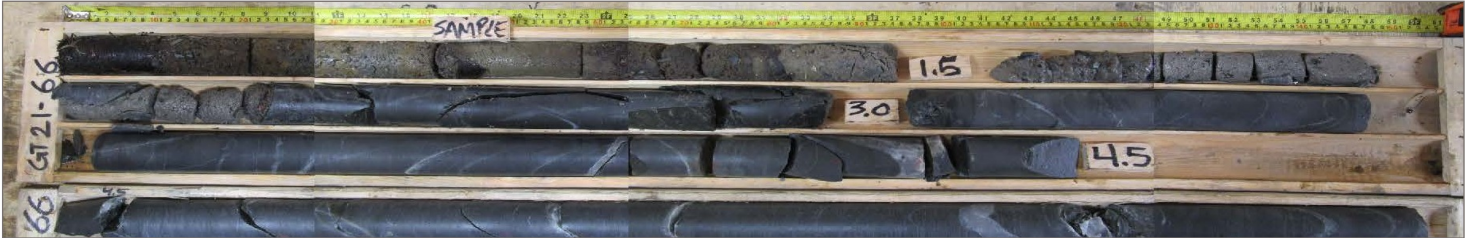
Photo 100: GT21-66 overburden & bedrock core; depth 0.0 – 5.93 m
