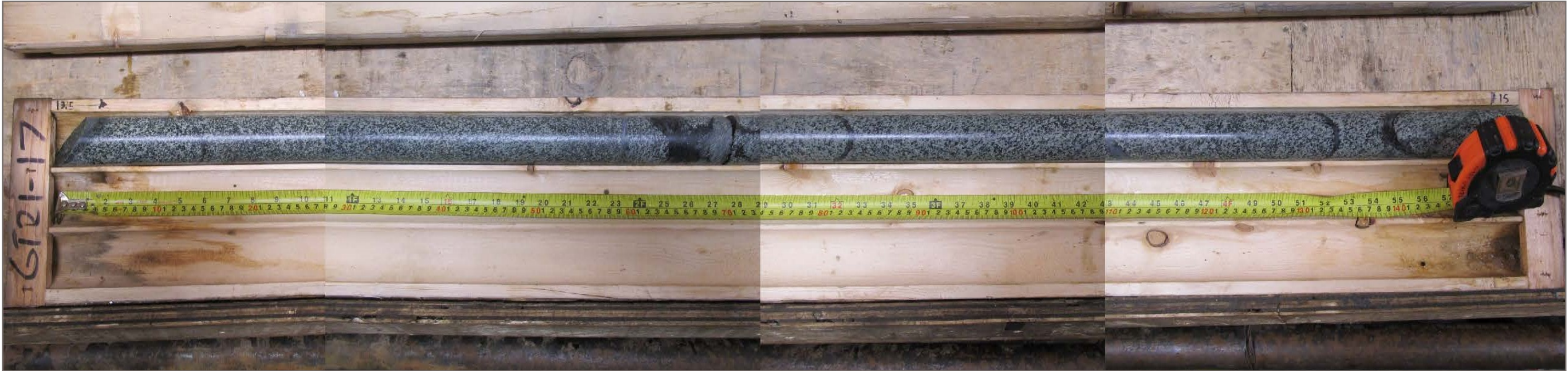
Photo 36: GT21-17 bedrock core; depth 13.5 – 15.0 m
