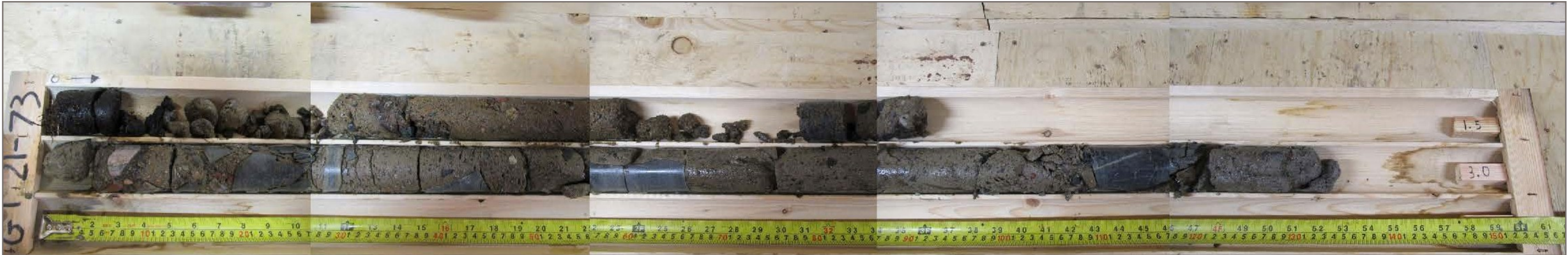
Photo 79: GT21-73 overburden core; depth 0.0 – 3.0 m
