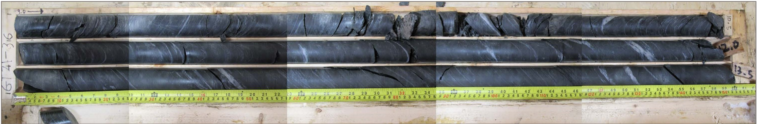
Photo 14: GT21-61 (36) bedrock core; depth 9.0 – 13.5 m
