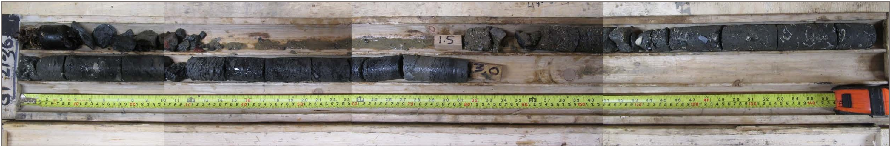
Photo 9: GT21-61 (36) overburden core; depth 1.5 – 3.0 m
