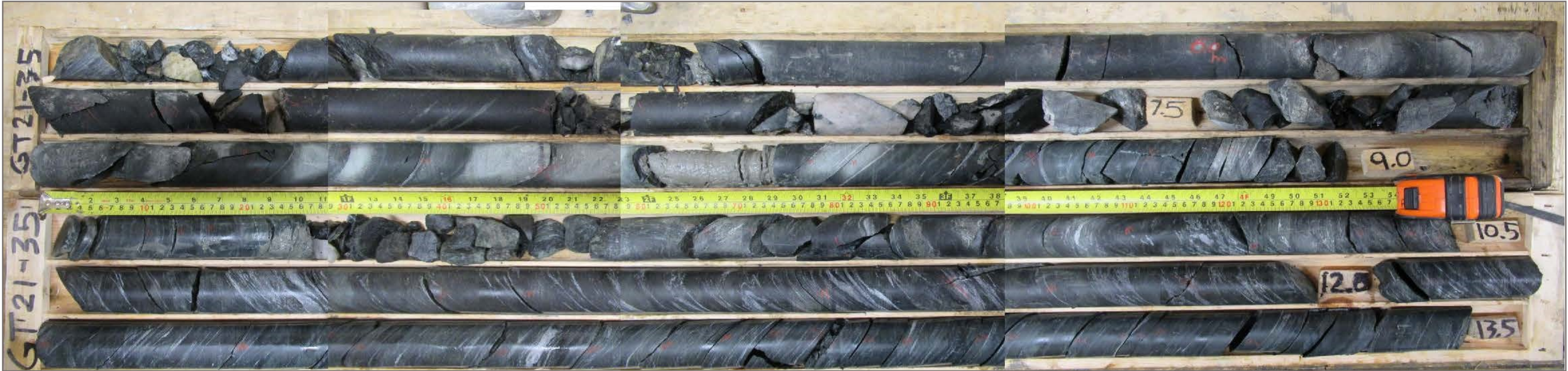
Photo 4: GT21-60 (35) overburden & bedrock core; depth 4.5 – 13.5 m
