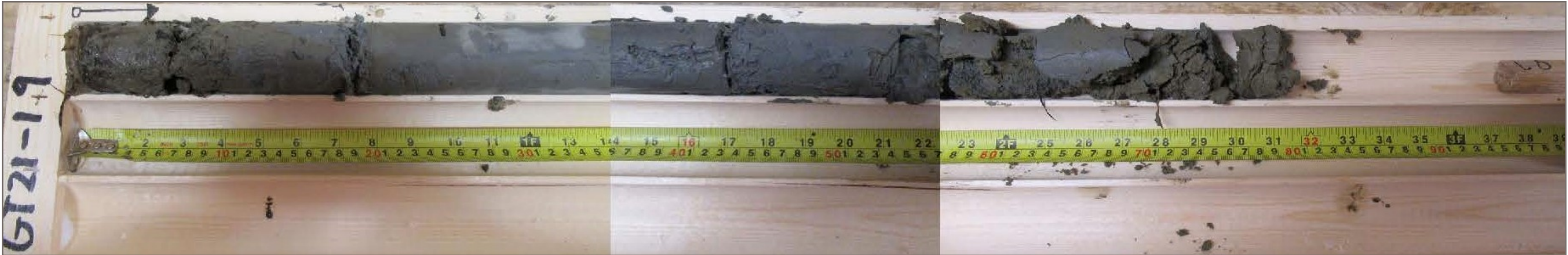
Photo 47: GT21-19 overburden core; depth 0.0 – 1.0 m
