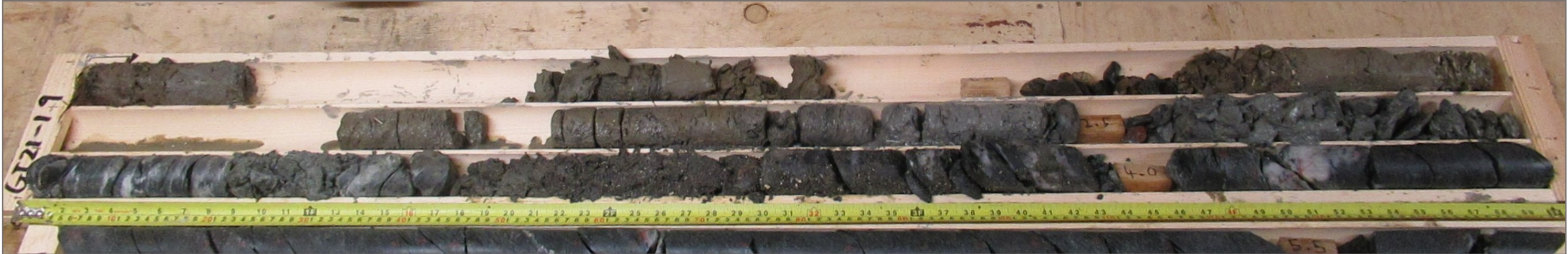
Photo 49: GT21-19 overburden & bedrock core; depth 2.5 – 4.36 m
