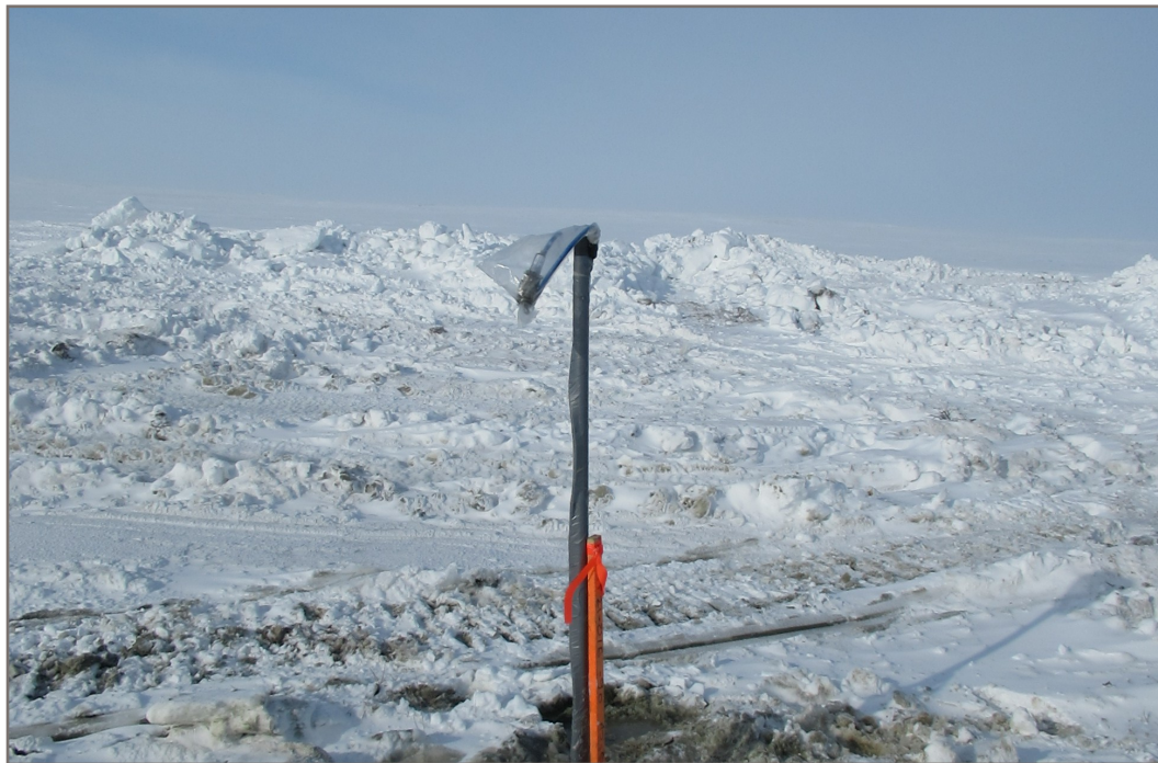
Photo 32: GT21-16 multi-bead GTC installation; depth 14.3 m
