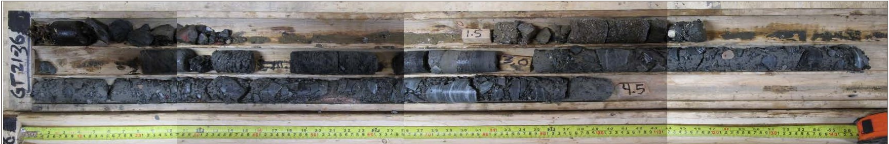
Photo 11: GT21-61 (36) overburden core; depth 3.0 – 4.5 m
