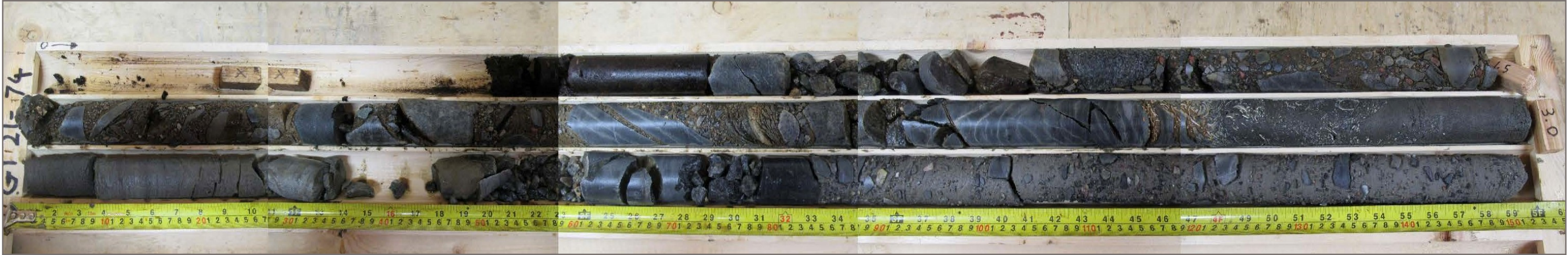
Photo 86: GT21-74 overburden core; depth 0.0 – 4.5 m
