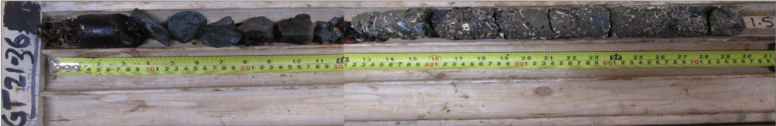
Photo 8: GT21-61 (36) overburden core; depth 0.0 – 1.5 m
