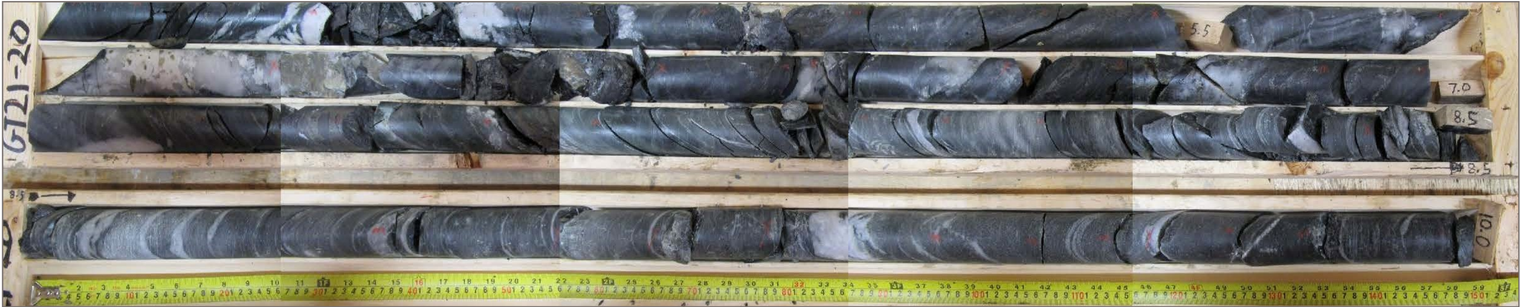
Photo 54: GT21-20 bedrock core; depth 4.14 – 10.0 m
