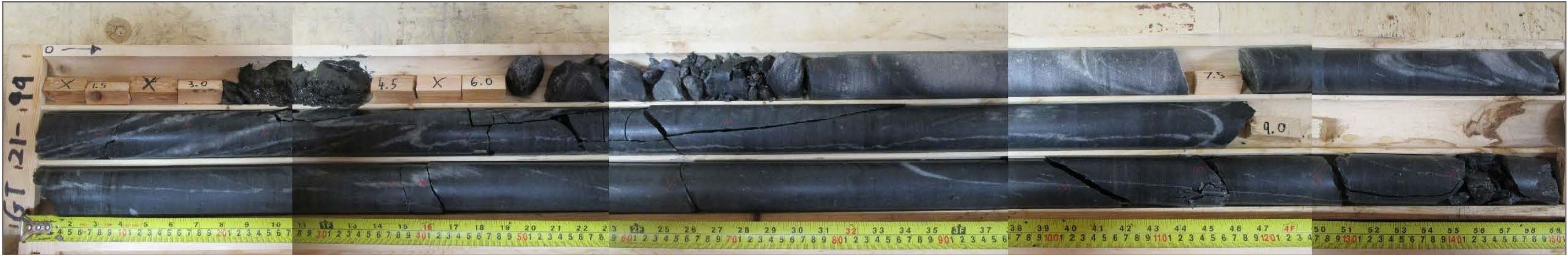
Photo 105: GT21-99 overburden & bedrock core; depth 0.0 – 10.5 m
