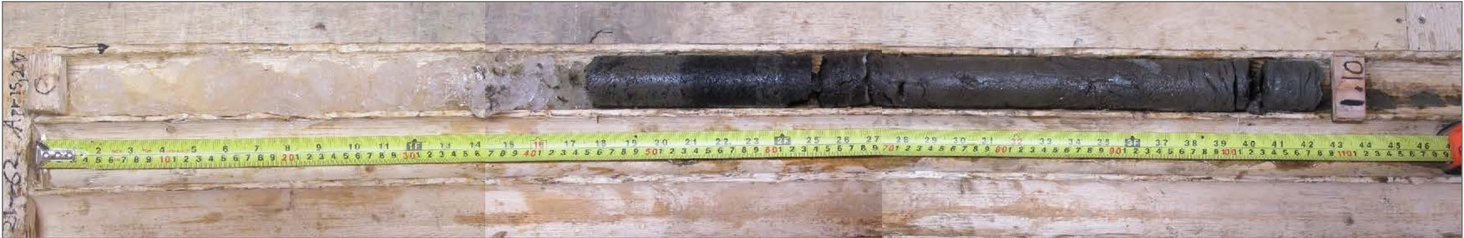
Photo 20 : GT21-62 (37) overburden core; depth 0.0 – 1.1 m
