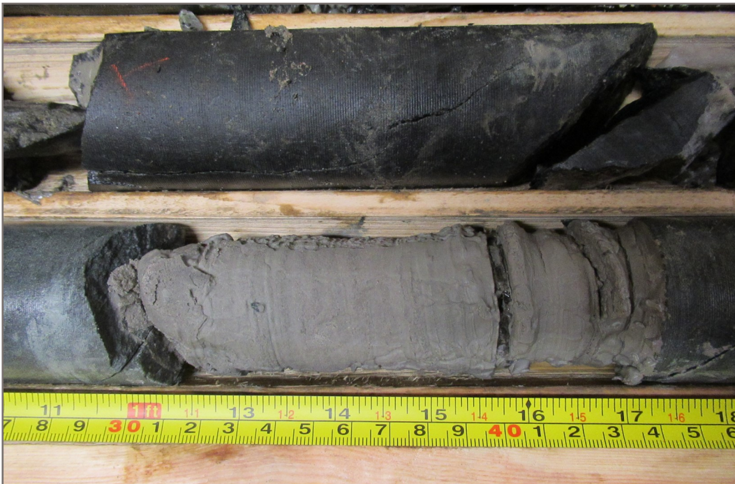
Photo 5: GT21-60 (35) overburden core; depth 8.3 m
