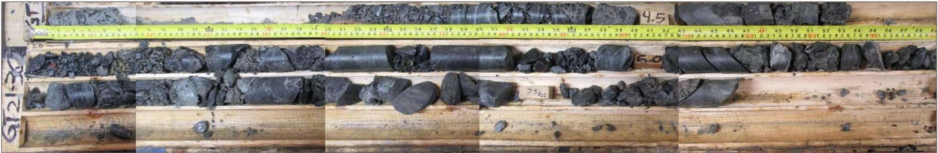
Photo 12: GT21-61 (36) overburden core; depth 4.5 – 7.5 m
