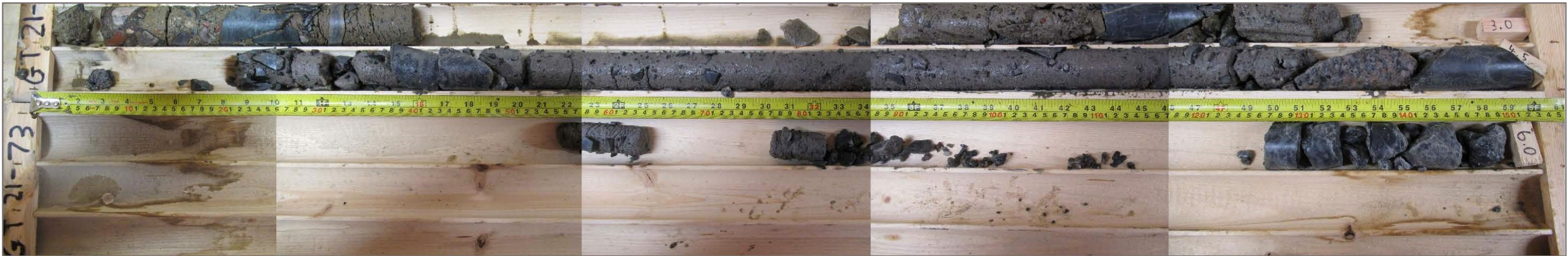
Photo 80: GT21-73 overburden core; depth 3.0 – 6.0 m
