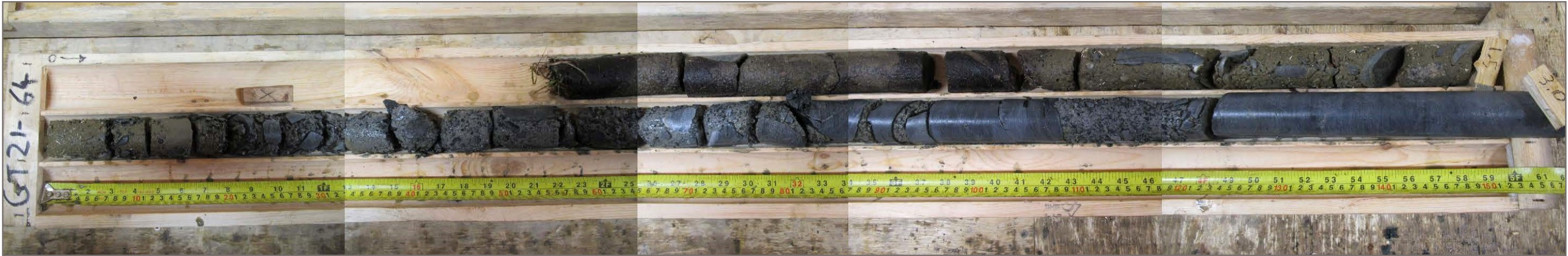
Photo 92: GT21-64 overburden & bedrock core; depth 0.0 – 3.0 m
