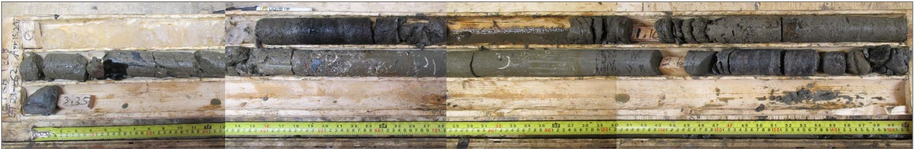
Photo 21 : GT21-62 (37) overburden core; depth 1.1 – 3.35 m
