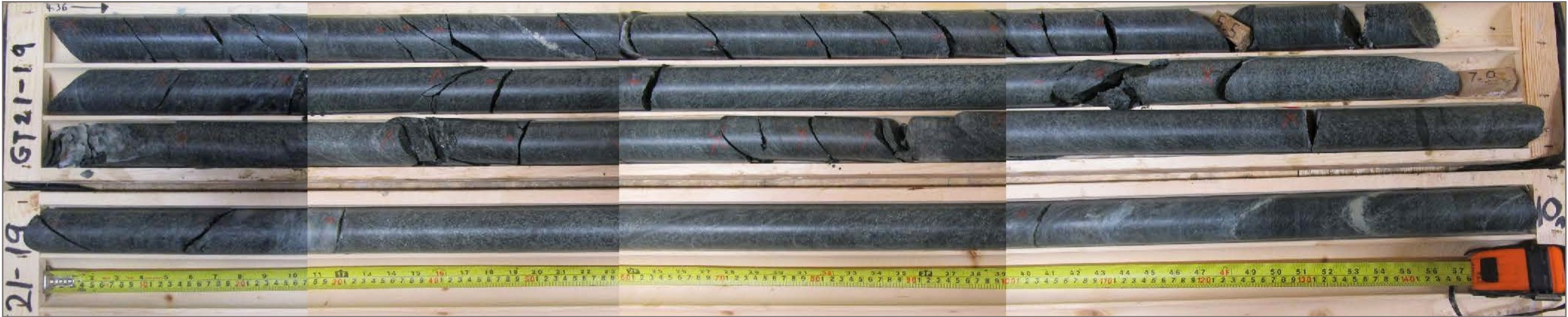
Photo 50: GT21-19 bedrock core; depth 4.36 – 10.0 m
