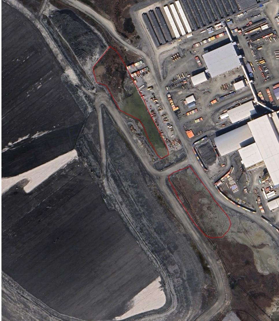
Figure 3.3-3: Proposed Areas to Store Frozen Tailings Material to Thaw until Final Deposition on TSF
