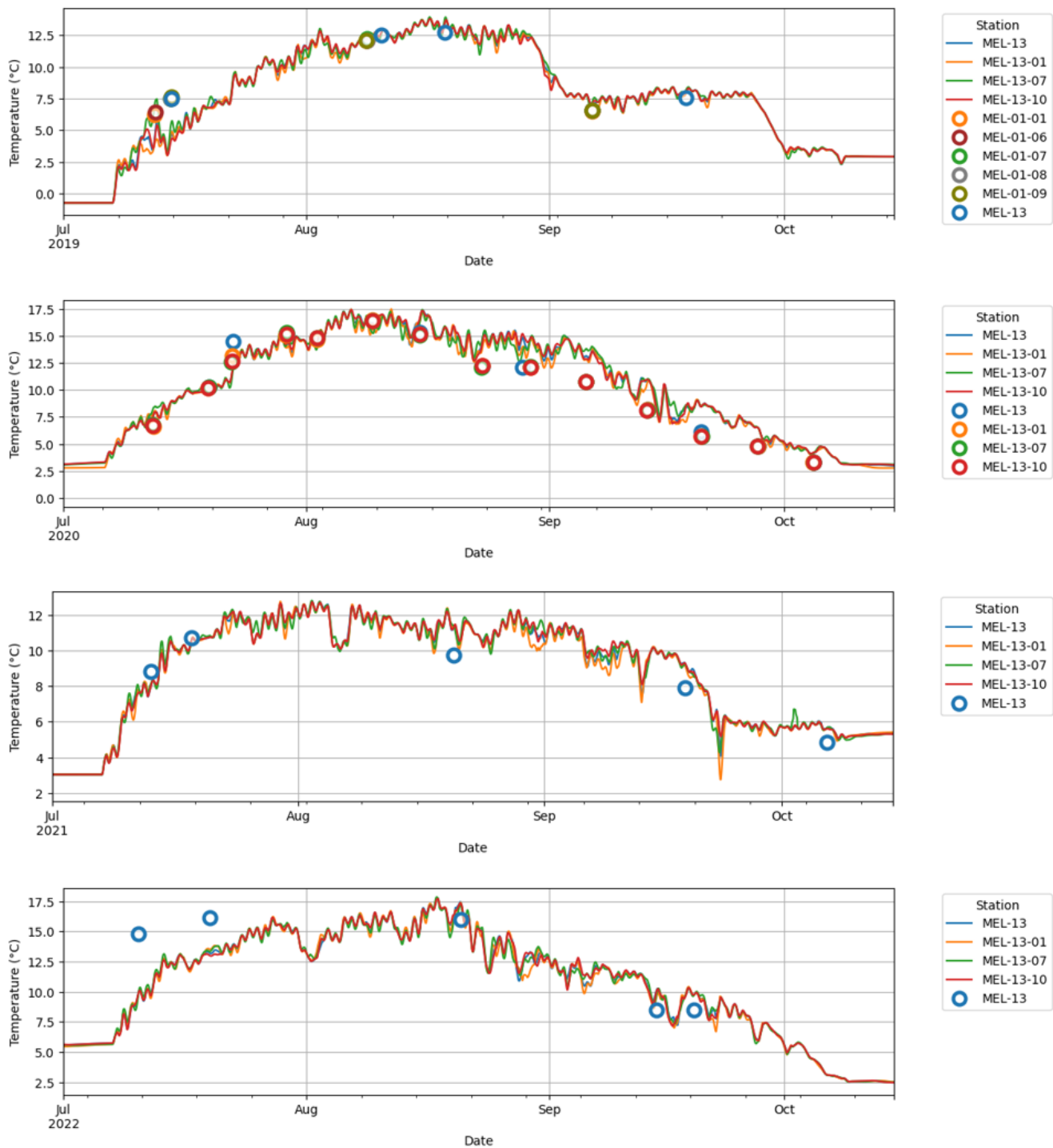
Figure A.3 Comparison of modeled and observed water temperature at monitoring stations near the diffuser for the 2019 to 2022 open-water season. Modeled results are shown as continuous lines, while observations at individual stations are shown as circles.
