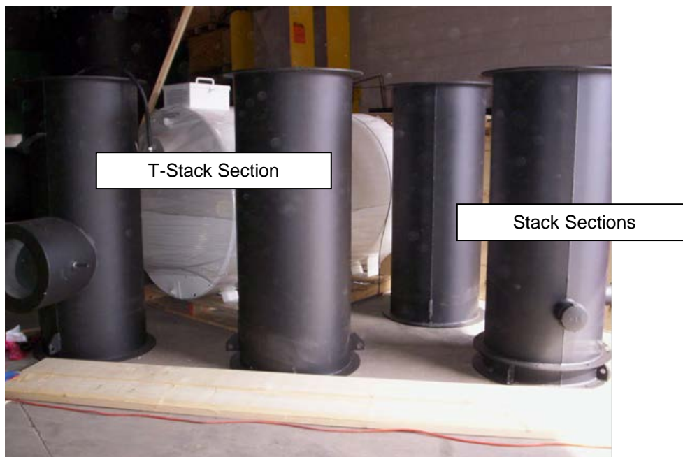
T-Stack and Stack Sections
