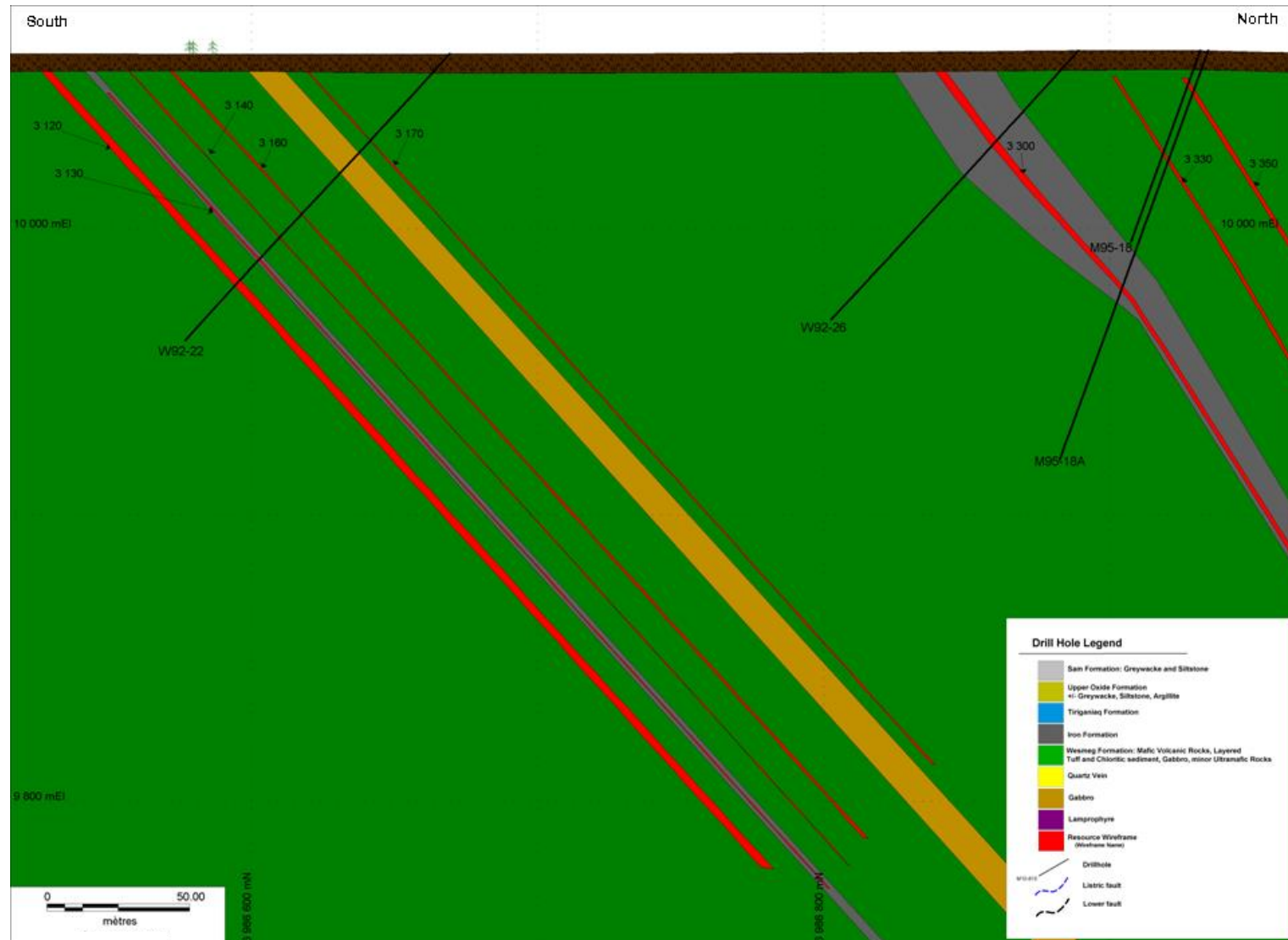
Figure 2-14 Pump Vertical Cross Section at 15,140 E (local grid) showing Geology and Lode Mineralization Solids
