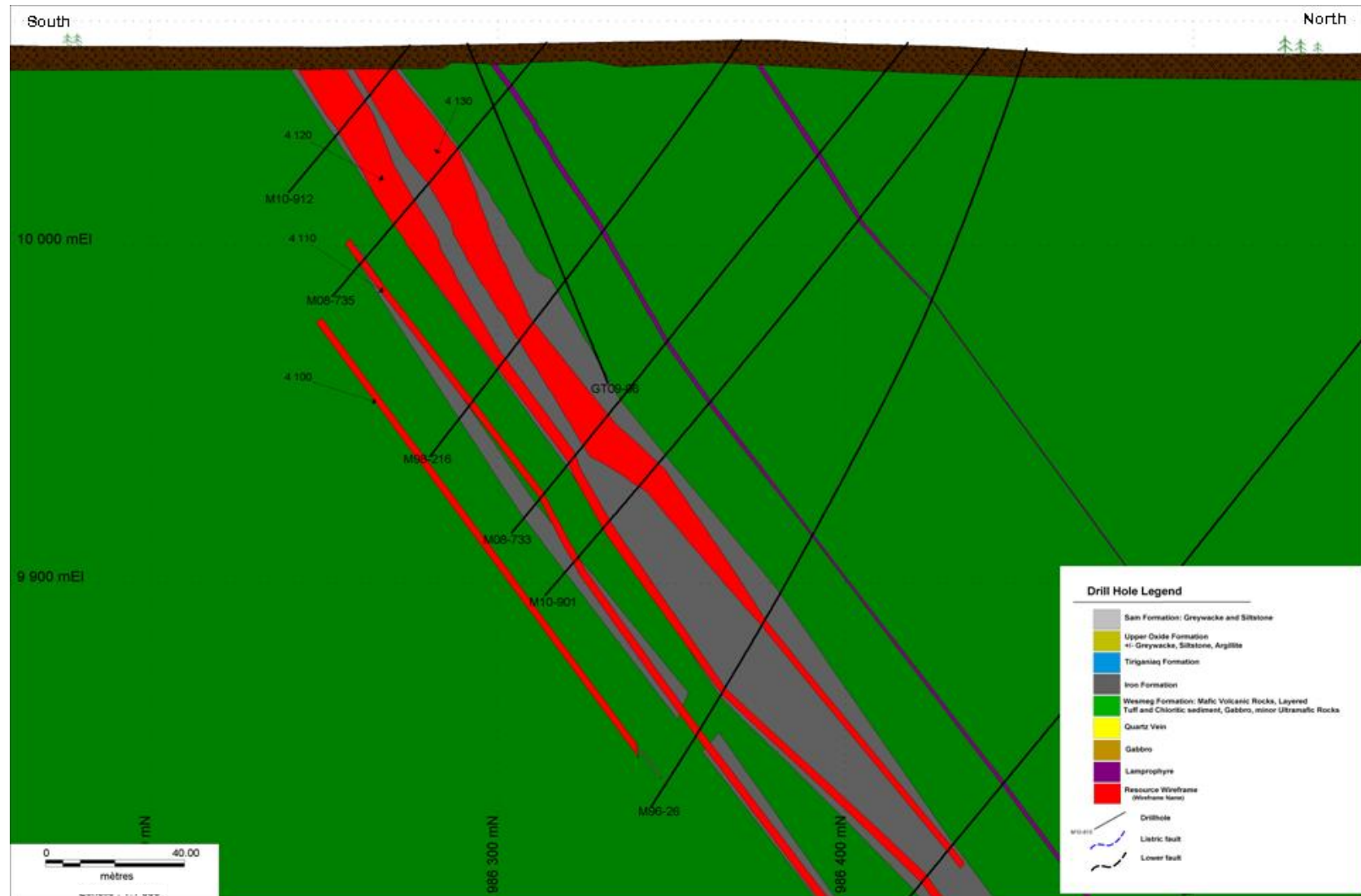
Figure 2-13 F Zone Vertical Cross Section at 17425 E (local grid) showing Geology and Lode Mineralization Solids
