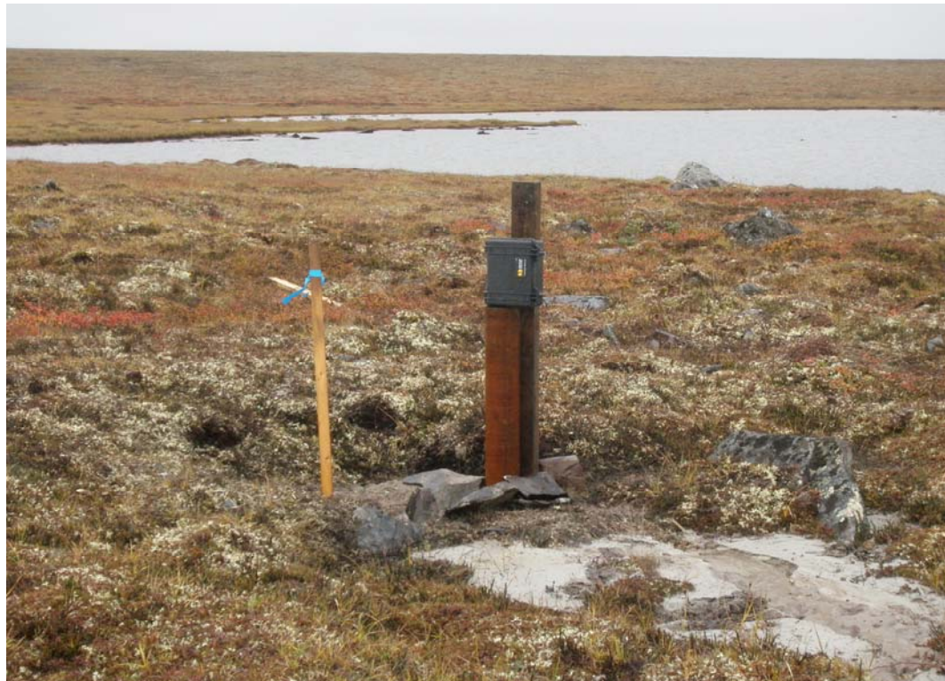
PHOTOGRAPH 4: Looking SE at GT11-07 Thermistor installation.
