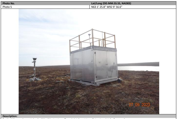
Partisol Air sampler contained within this structure. Two air intakes at top of structure intake for samplers.
