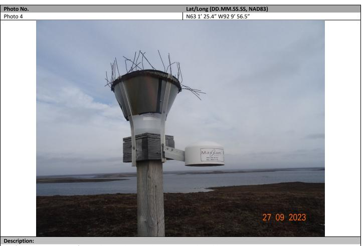
Dustfall collection jar on top of post with NO2 and SO2 sampler mounted on side in while canister.
