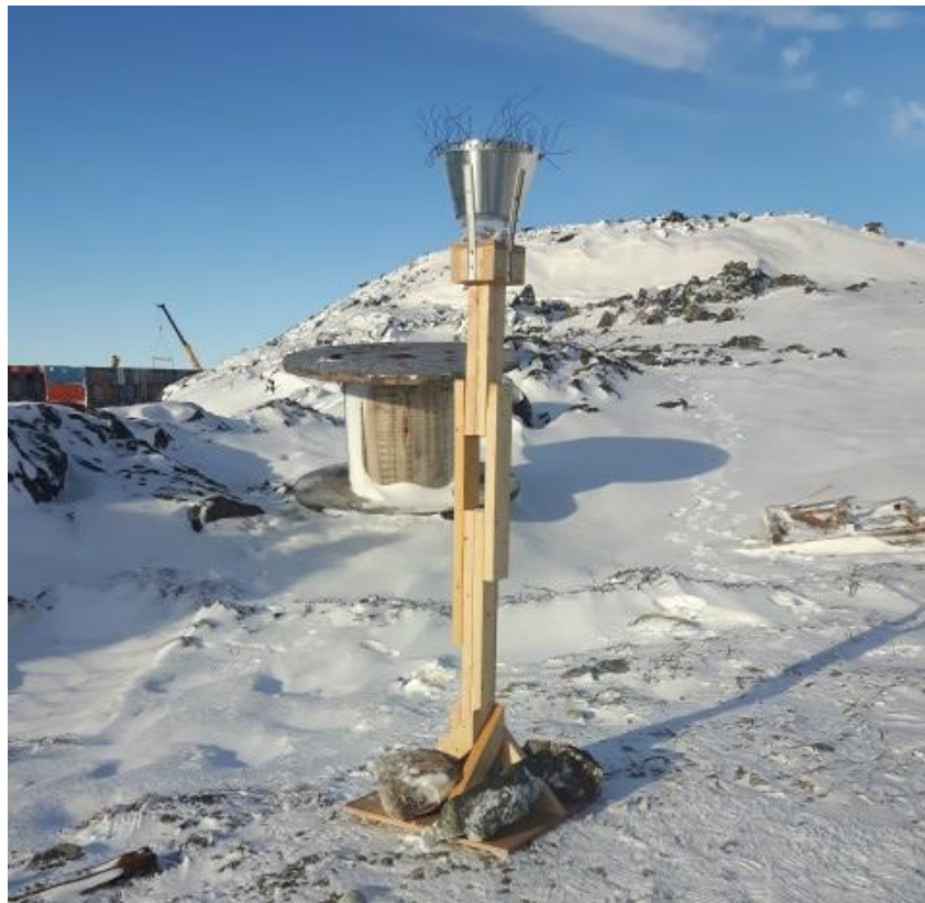
Figure 2. Dustfall sampling stand at the Meliadine site.
