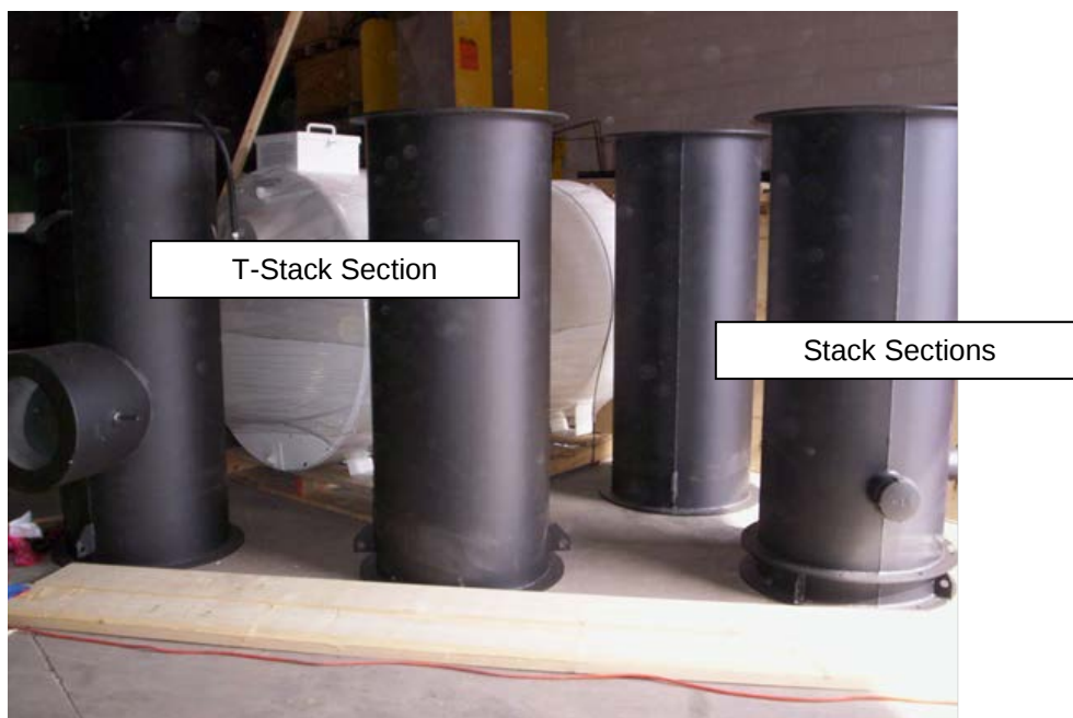
T-Stack and Stack Sections
