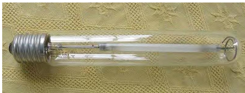
Figure 3 – High Pressure Sodium Discharge Lamp
