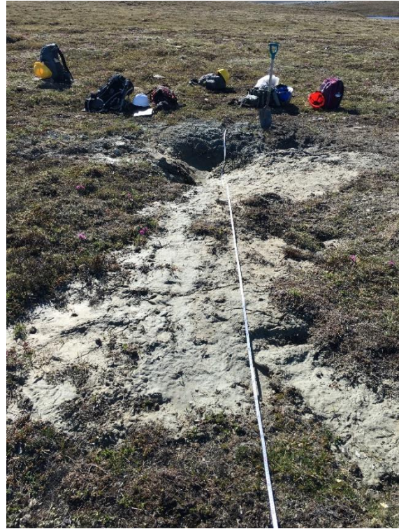
Figure 5. Larger patches of drilling waste evident at the surface on newer drilling sites (left M12-1863; right M17-2398).
