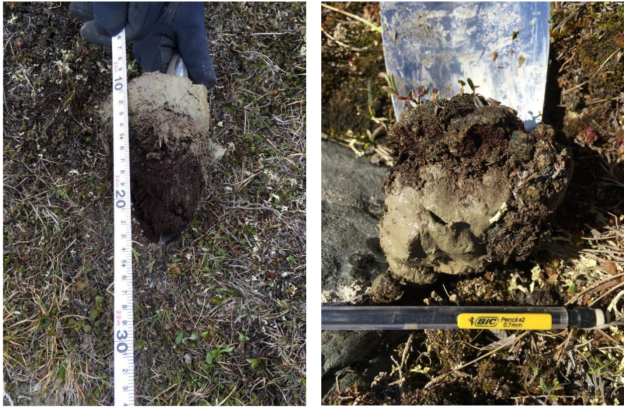
Figure 10. Drilling waste ~3 cm in depth underlain by an organic soil horizon (left) and organic matter accumulation over drilling waste (right).
