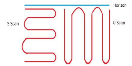
Figure D-4: S and U scanning techniques
