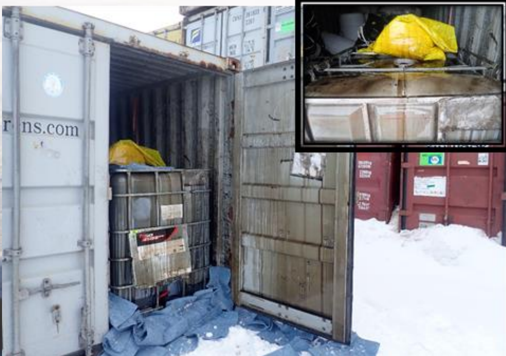
Tote Placed in Seacan without a Cap Resulted in an Oil Spill
