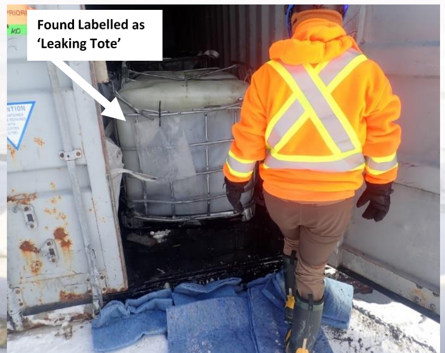
Leaking Tote Placed in Seacan Resulted in an Oil Spill
